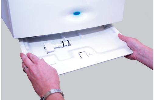
In the case of the keyed filling link, it is necessary to locate the key (see above). Remove the bottom panel by pulling the catch down and then pulling the panel forward and down to remove. If the key is displaced you may order a spare key by calling customer service: 0330 123 9559.
