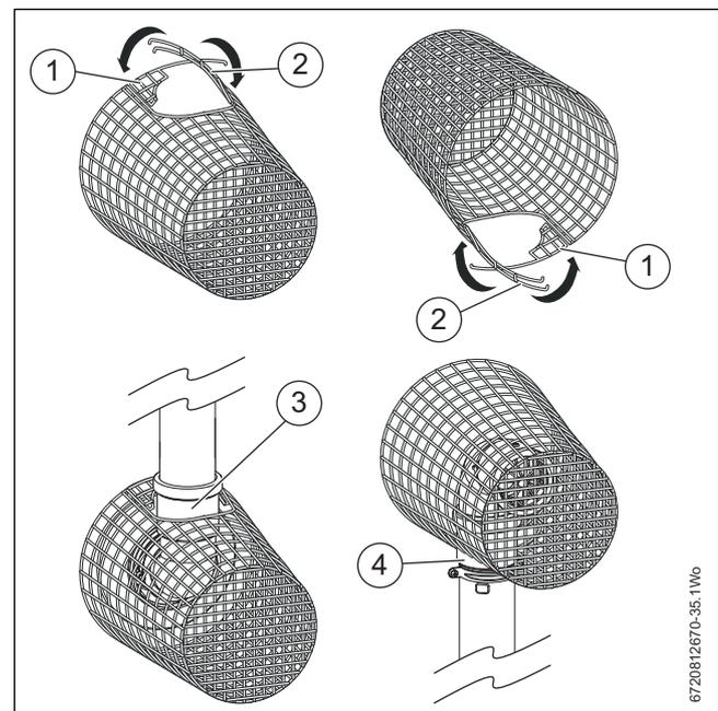
Fig. 37 Fitting terminal guard
