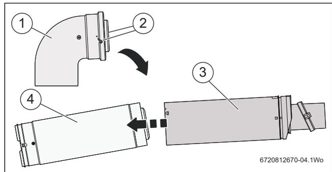
Fig. 10 Separating elbow from telescopic flue
