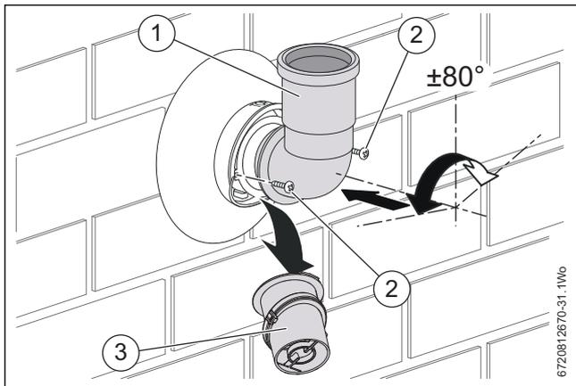
Fig. 33 Plume management terminal bend
