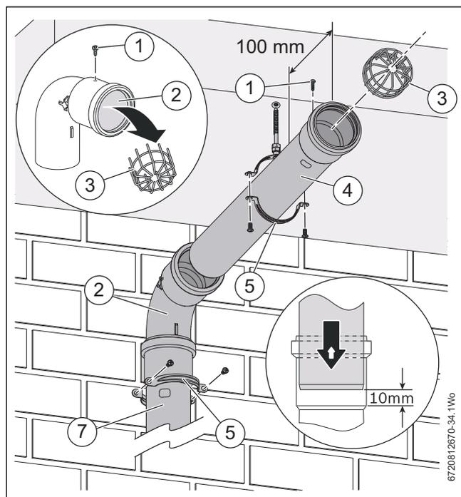
Fig. 36 Fitting extension under balcony/overhang
