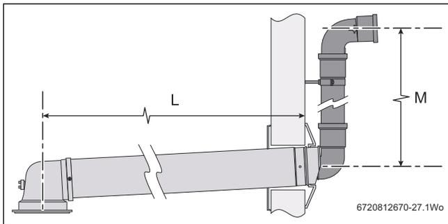
Fig. 29 Effective lengths determination
