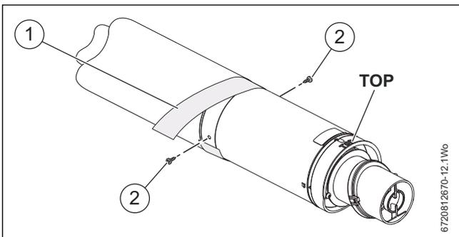
Fig. 13 Setting the telescopic flue length
