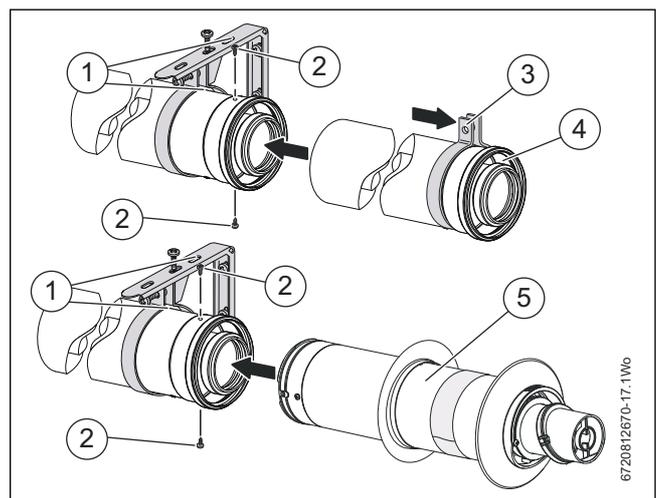
Fig. 18 Extension and telescopic flue connection examples
