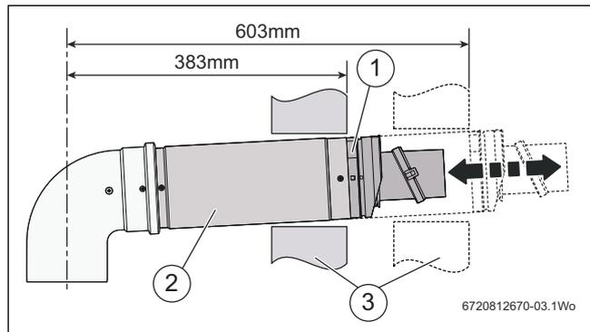
Fig. 9 Standard telescopic flue lengths
