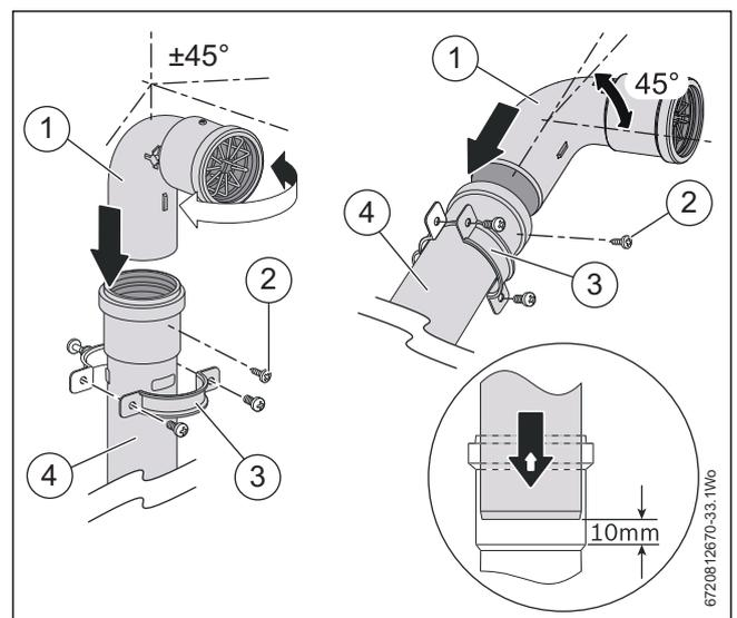
Fig. 35 Fitting the discharge elbow
