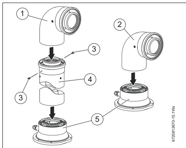
Fig. 16 Connection to the flue adaptor examples
