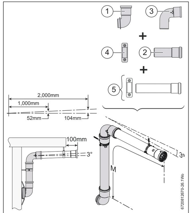
Fig. 28 Extended under a balcony/overhang option
