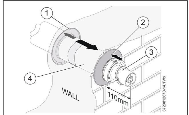
Fig. 14 Telescopic flue through the wall
