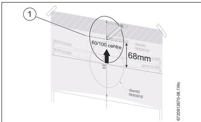
Fig. 5 Adjusted 60/100mm flue exit hole
