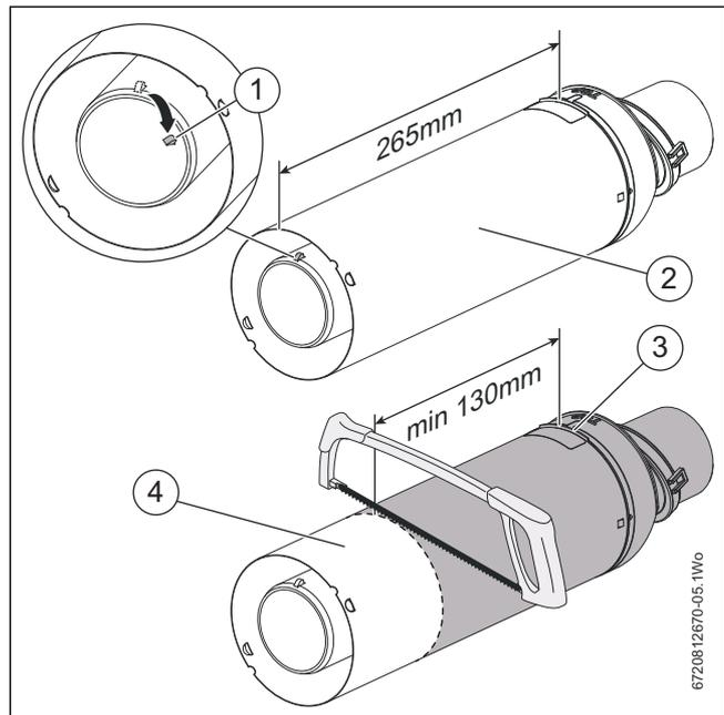
Fig. 11 Shortening the terminal assembly
