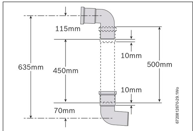
Fig. 31 Plume management 90° bends offset example
