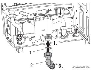
Fig. 30 Condensate connections
