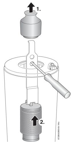
Fig. 62 Baffle removal
