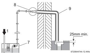
Fig. 13 Condensate pump to external disposal
