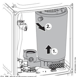
Fig. 88 Heat exchanger removal
