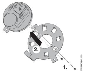
Fig. 77 Air pressure switch bracket
