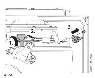
► Undo the securing nut at the top of the heat exchanger and remove the retaining plate assembly (1).
