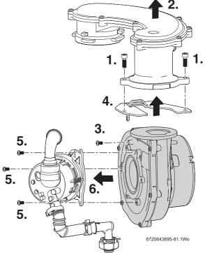
Fig. 78 Dismantling the air/gas manifold assembly
