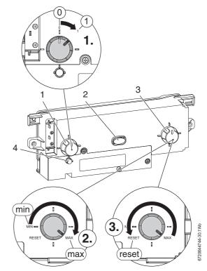
Fig. 41 Boiler controls
