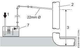
Fig. 10 Condensate pump disposal
