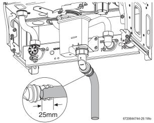
Fig. 39 Condensate connection
