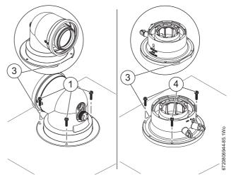
Fig. 33 Flue turret/adaptor connection
