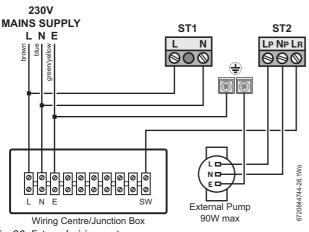
Fig. 36 External wiring centre
