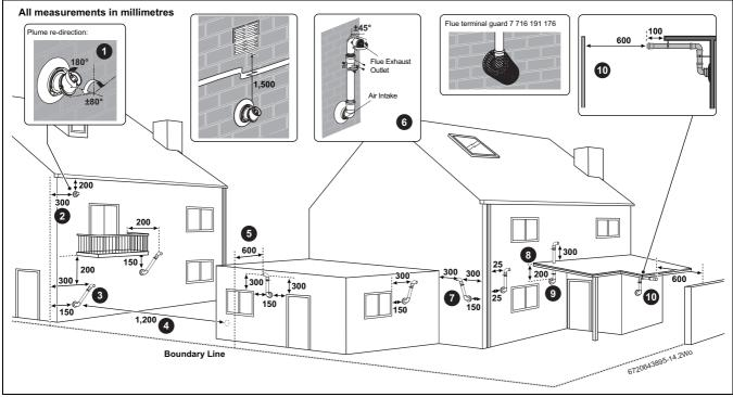
Fig. 21 Plume terminal positions
