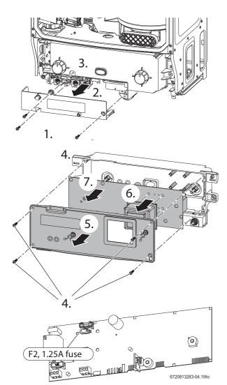
Fig. 91 Transformer/PCB/Fuse access
