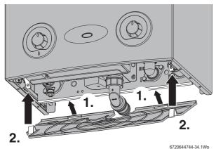
Fig. 66 Remove bottom panel
