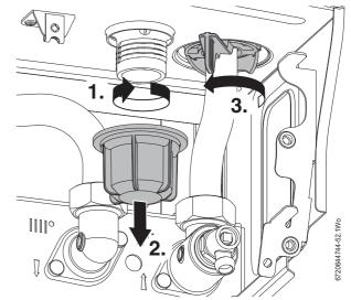
Fig. 87 Sump connections
