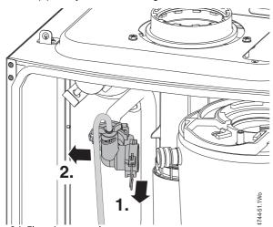
Fig. 84 Flow pipe removal
