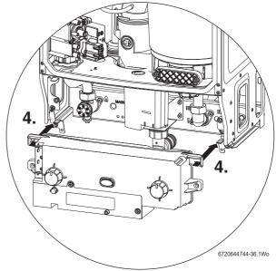
Fig. 71 Control panel into service position
