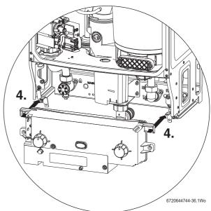
Fig. 49 Control panel into service position
