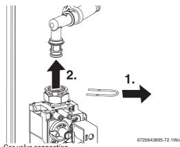
Fig. 58 Gas valve connection
