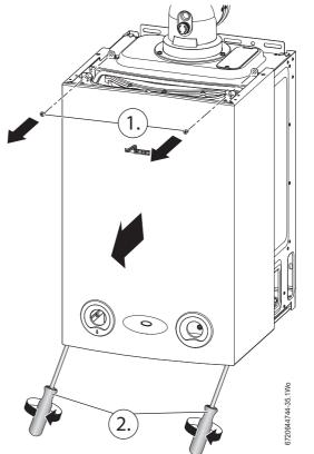
Fig. 48 Remove outer case
