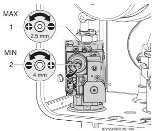
Fig. 57 Gas valve adjustment
