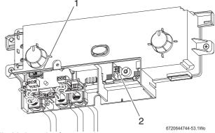
Fig. 90 Removing the connection cover
