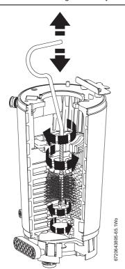
Fig. 64 Cleaning heat exchanger
