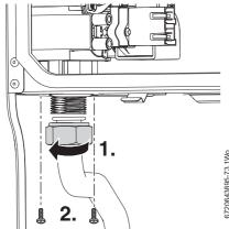
Fig. 73 Gas valve lower connection
