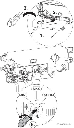
Fig. 52 Setting the boiler to maximum
