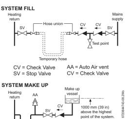
Fig. 2 System fill/System make-up
