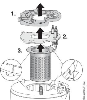
Fig. 80 Electrode assembly and burner
