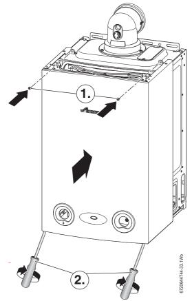
Fig. 46 Replacing outer case
