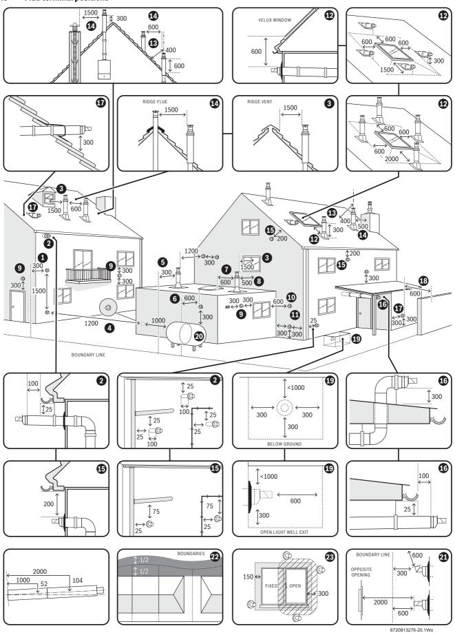
Fig. 20 Flue terminal positions
