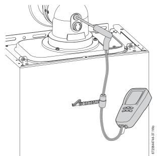
Fig. 51 Flue integrity test
