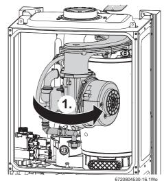
Fig. 75 Rotate the air/gas manifold assembly
