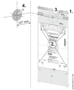
Fig. 26 Marking the flue position
