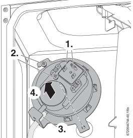
Fig. 76 Air pressure switch
