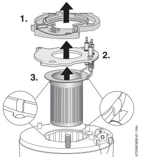
Fig. 61 Burner removal
