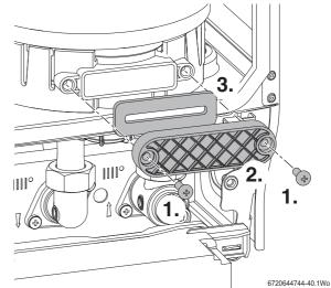
Fig. 63 Access cover removal
