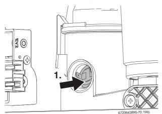
Fig. 70 Remove thermostat
