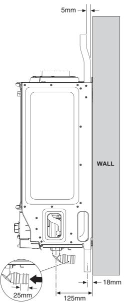
Fig. 31 Pipe work dimensions
