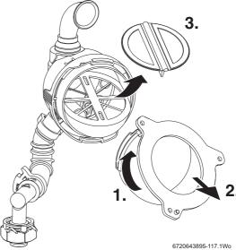
Fig. 79 Flap valve assembly
