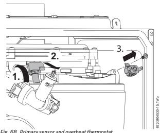
Fig. 68 Primary sensor and overheat thermostat
