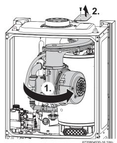
Fig. 60 Rotate air/gas manifold
