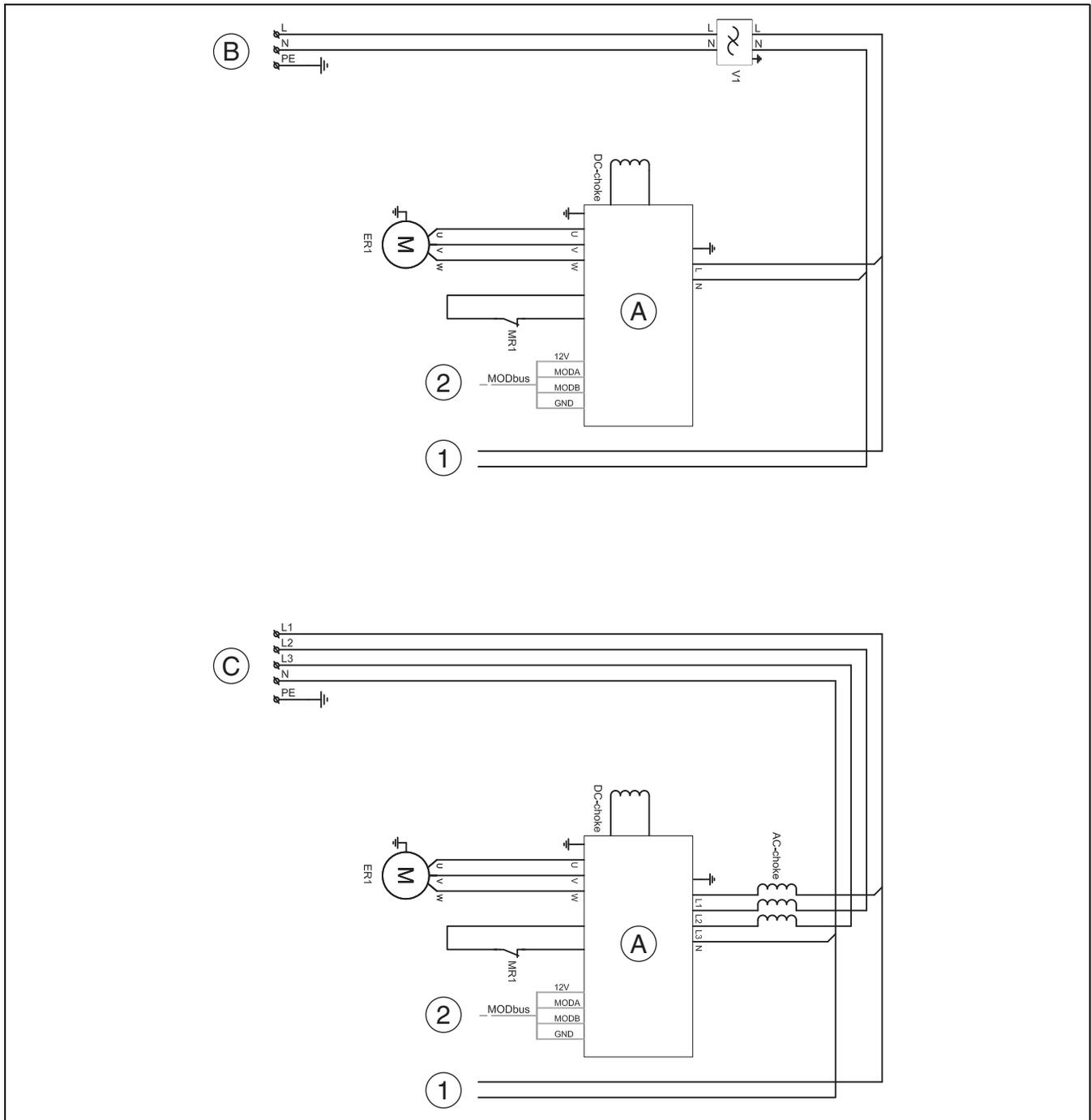
Fig. 25 Wiring diagram for transformer, alternating current / three-phase current
