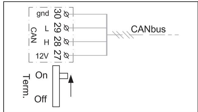
Fig. 19 Termination CAN-BUS
