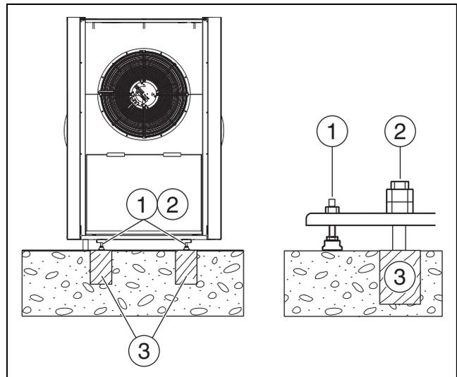
Fig. 14 Fastening the heat pump
