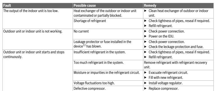
1) A fuse for the overcurrent protection is located on the main PCB. The specification is printed on the main PCB and can also be found in the technical data on page 60. Use only ex-protected ceramic fuses.
