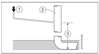
Fig. 11 Disposal to soil vent stack
