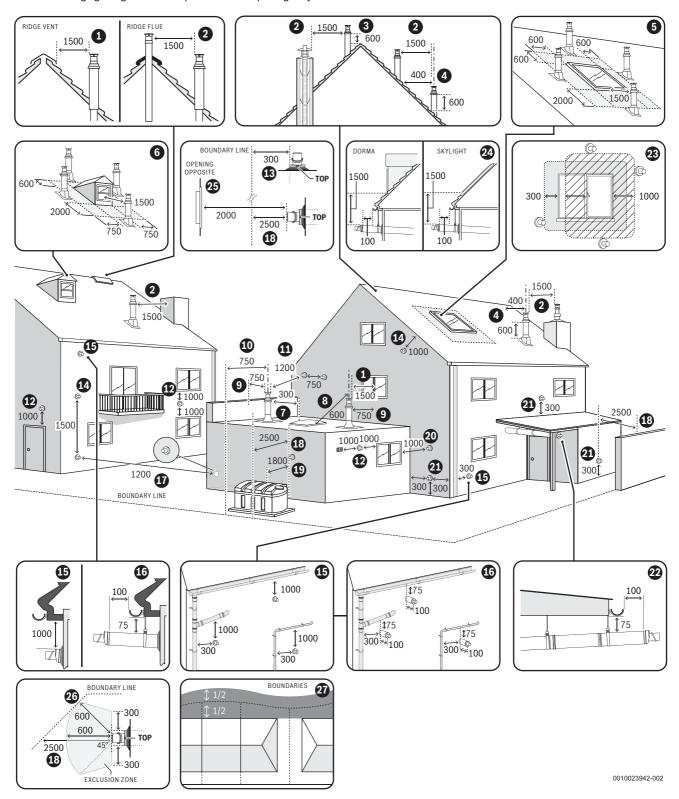
Fig. 24 Flue terminal positions
