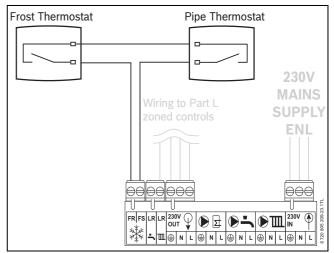
Fig. 50 Optional External 230 V AC Frost Stat Connection for protection of system pipework in unheated air space
