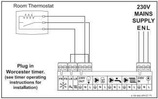
Fig. 49 Room Thermostat and Plug In Twin Channel Programmer
