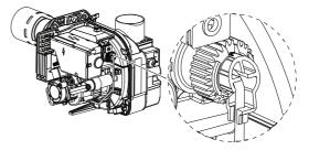
Fig. 63 Burner head adjustment thumbwheel
