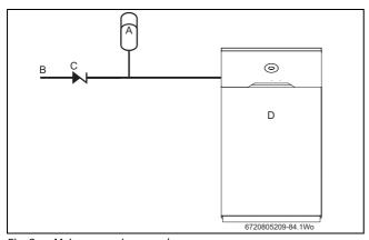
Fig. 3 Mains expansion vessel
