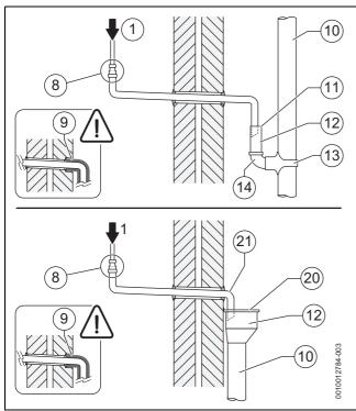
Fig. 15 Disposal into a rainwater down pipe
