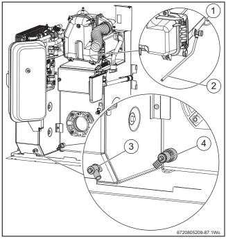
Fig. 78 Appliance drains points
