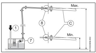
Fig. 13 Condensate pump disposal
