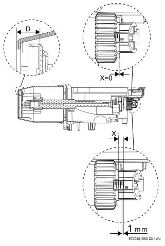
Fig. 64 Burner head adjustment
