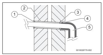
Fig. 14 Additional protection for transition through a walll
