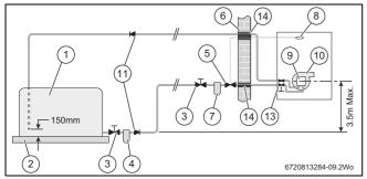
Fig. 5 Double pipe feed
