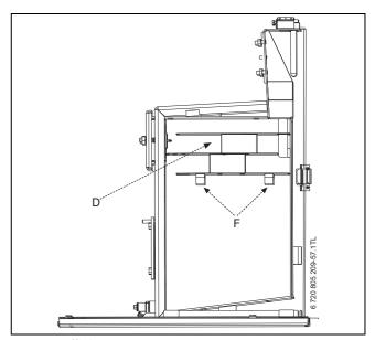
Fig. 90 Baffle location
