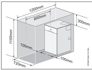
Fig. 20 Installation clearances
