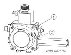
Fig. 86 Pump filter access
