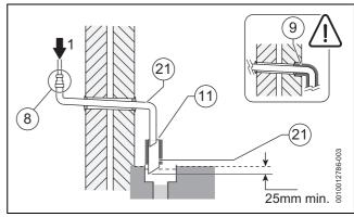
Fig. 16 Disposal to open drain or gully with air break
