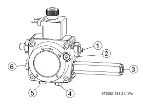
Fig. 104 Oil pump ports/connections
