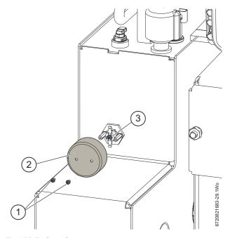
Fig. 106 Tank overheat reset
