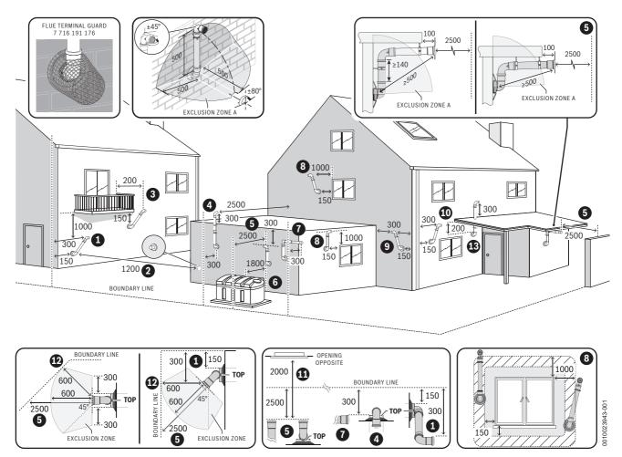
Fig. 27 Plume terminal positions
