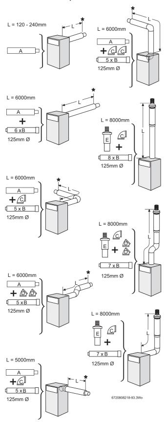
Fig. 26 Room sealed flue options
