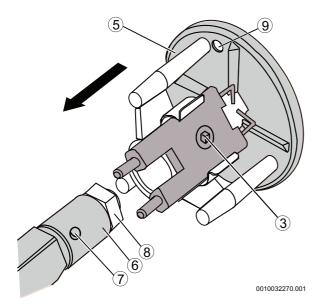
Fig. 84 Photocell alignment
