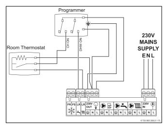
Fig. 48 External 230 V Twin Channel Programmer and Room Thermostat
