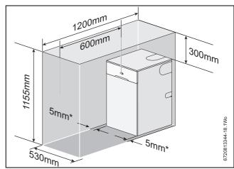
Fig. 22 Maintenance and repair clearances
