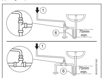
Fig. 12 Disposal to a waste pipe
