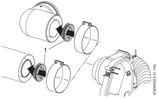
Fig. 34 Flue damper fitting
