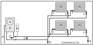
Fig. 8 Combi boiler sealed system layout
