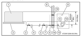
Fig. 4 Single pipe feed
