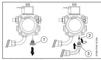
Fig. 42 Converting to double pipe system
