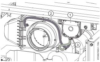
Fig. 107 Sensing tube connections
