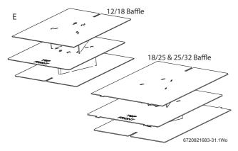
Fig. 89 Baffle arrangement
