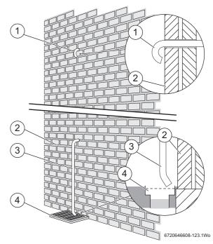
Fig. 19 Pressure relief pipe work
