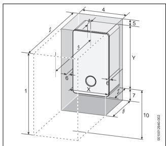
Fig. 7 Appliance minimum clearances
