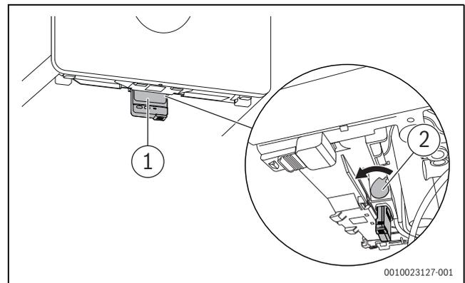
Fig. 7 Locking mechanism
