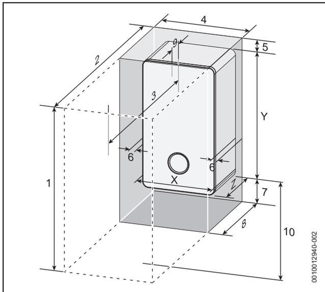
Fig. 8 Appliance minimum clearances
