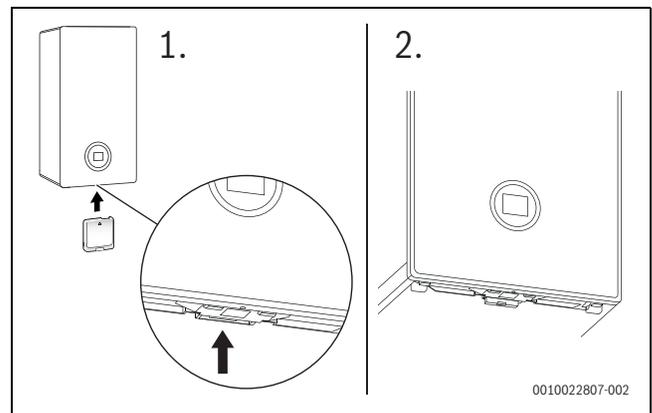
Fig. 6 Position of Key housing
