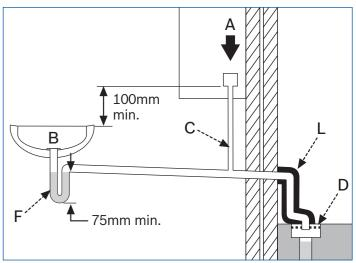
Internal waste drainage system
