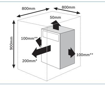
\*Space required for unvented areas with a removable door or panel. \*\*This space can be reduced to 50mm for one side only as along as both the side clearances add up to the total of both the side measurements shown or more.
