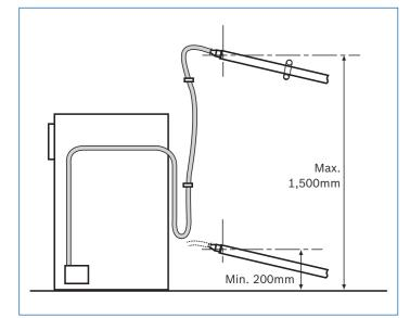
• The flexible plastic pipe can be reduced in length to suit the installation circumstances. The pipework must follow one of the options shown opposite.
