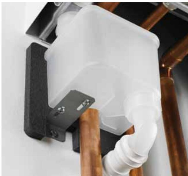
CondenseSure clips onto the 22mm heating flow pipe using the 'free' heat to raise the condensate temperature.
