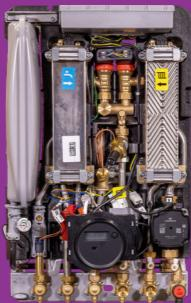
Two heat exchangers – one for providing instant domestic hot water (DHW) at a regulated temperature and another for space heating (CH) within the property. The primary heating circuit is hydraulically separated from the property by both plate heat exchangers, providing higher security from district leaks.
