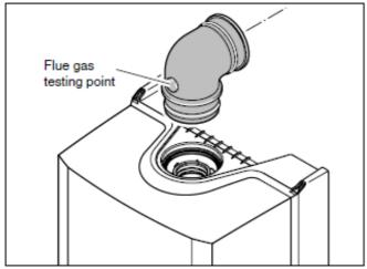
Fig 2: Flue sampling point
