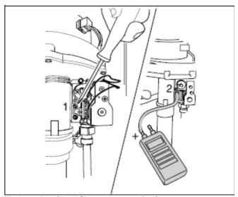
Fig 3: setting the Air/Gas ratio control valve
