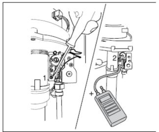
Fig 1: Inlet test nipple for the SIT gas valve
