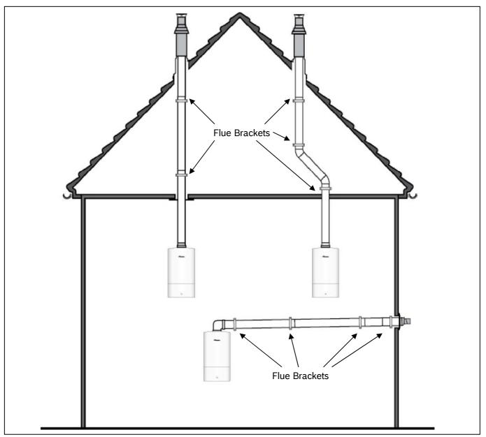
*Fig. 1: example of flue supports*
