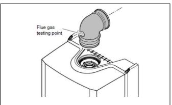
Fig 1: Flue test point
