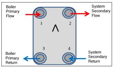
Fig. 1 Plate Heat Exchanger orientation & connections
