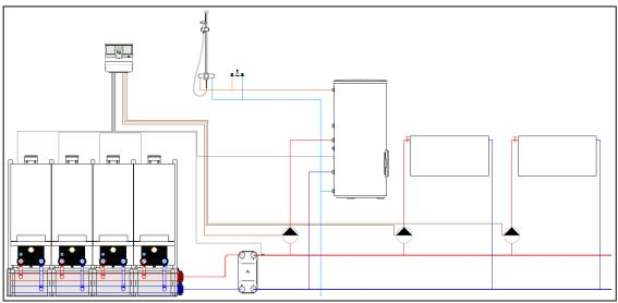
Fig. 2 Example plate heat exchanger system layout
