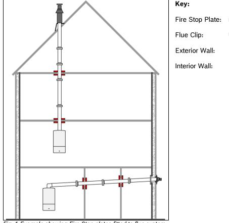
Fig. 1 Example showing Fire Stop plates fitted to flue system.
