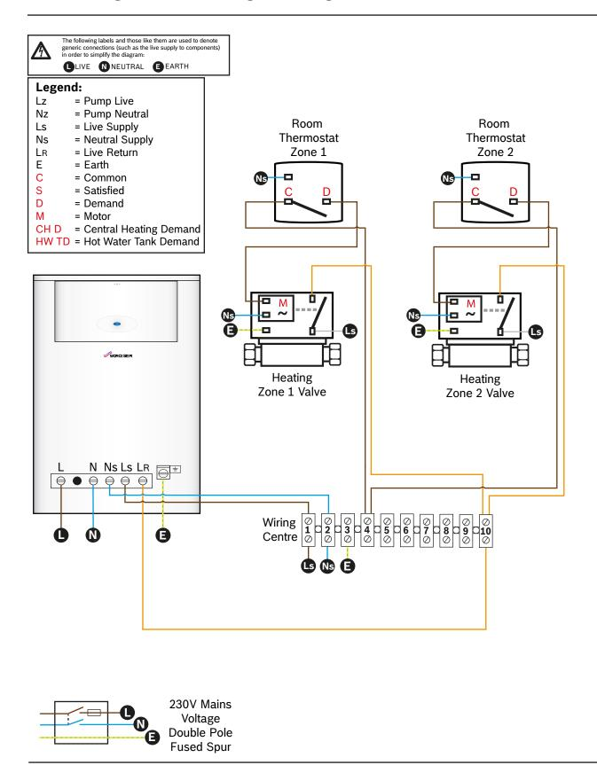
All electrical work should be carried out by a registered engineer. Wiring must comply with the latest IET wiring regulations. Isolate the mains electricity supply before starting any work and observe all relevant safety precautions. Refer to all relevant product installation manuals for safety and installation instructions
