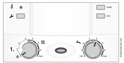
Fig. 3 Switch off central heating
