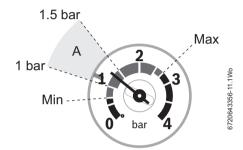
Fig. 6 Optimum pressure when cold (area A)
