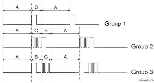
Fig. 104 Fault flash timing
