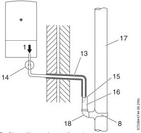
Fig. 7 Disposal into a rainwater down pipe
