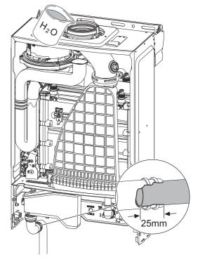
Fig. 31 Connecting and filling the siphon
