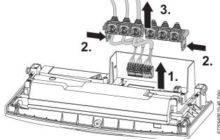
Fig. 102 Cable removal
