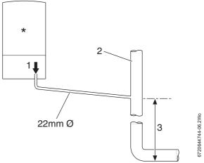
Fig. 4 Disposal to soil vent stack
