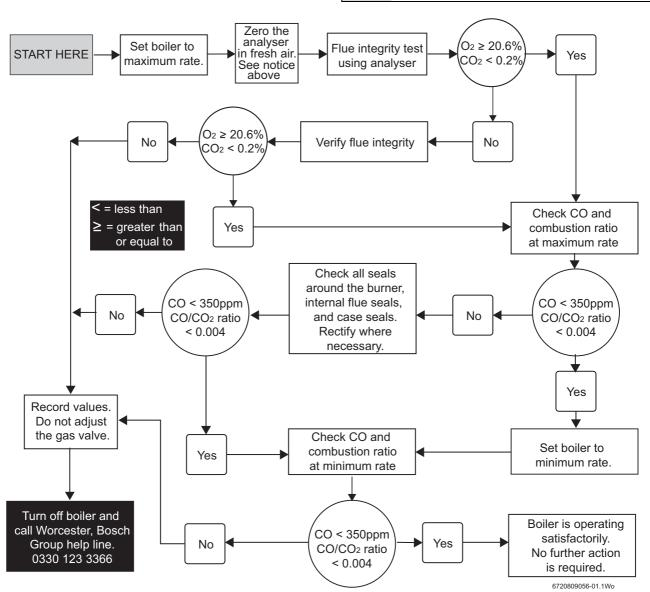
Fig. 58 Combustion check flow chart
