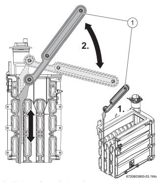
Fig. 73 Heat exchanger cleaning tool
