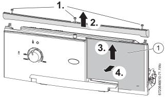
Fig. 45 Removing the blanking plate
