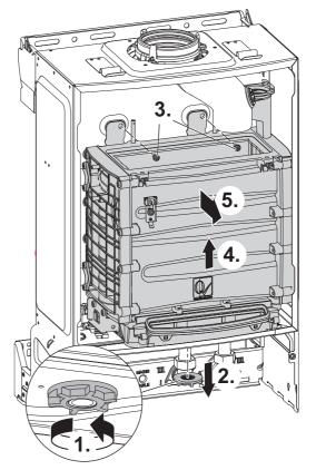
Fig. 98 Heat exchanger removal
