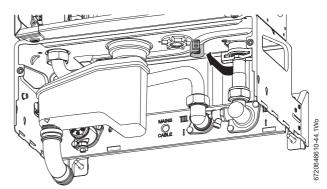
Fig. 99 Boiler return sensor
