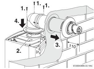
Fig. 39 Telescopic flue installation
