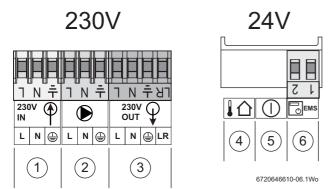
Fig. 44 230V and 24V connections
