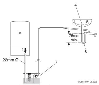
Fig. 6 Condensate pump disposal
