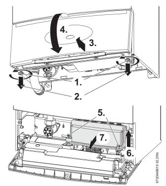
Fig. 53 Control panel to service position
