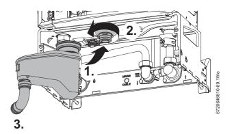
Fig. 71 Fitting siphon
