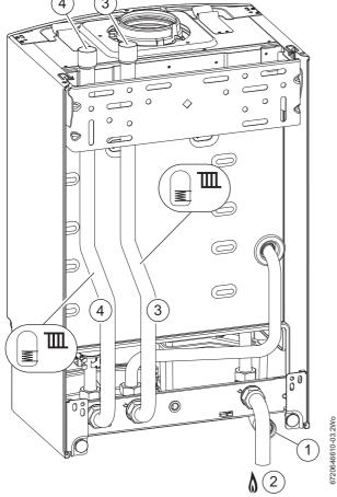
Fig. 14 Plumbing manifold
