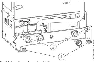
Fig. 30 Levelling and securing detail
