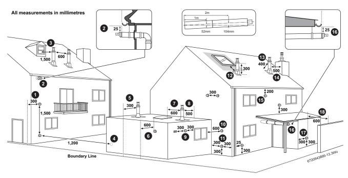
Fig. 15 Flue terminal positions
