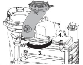
Fig. 89 Fan removal 1
