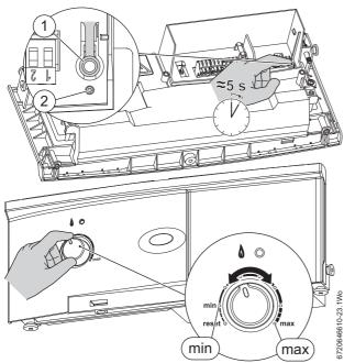
Fig. 65 Setting boiler to maximum
