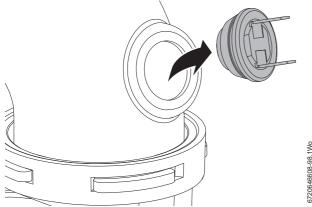
Fig. 81 Flue overheat thermostat
