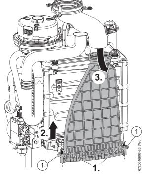
Fig. 84 Flueway removal
