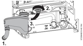
Fig. 78 Siphon removal
