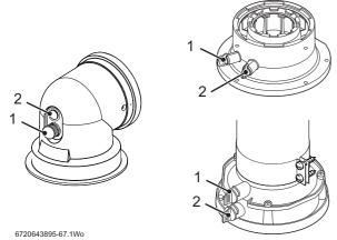
Fig. 62 Flue turret test points
