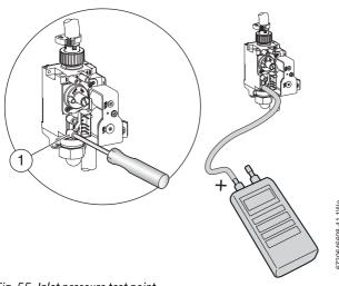
Fig. 55 Inlet pressure test point
