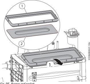
Fig. 95 Burner and gasket
