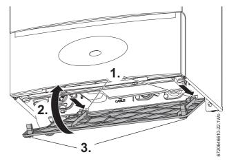
Fig. 61 Bottom panel installation
