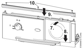
Fig. 47 Fitting the Programmer/Timer
