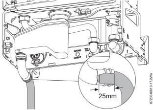
Fig. 51 Condensate connection
