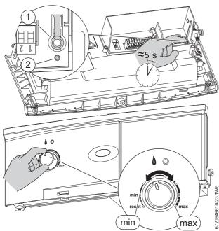
Fig. 68 Setting boiler to maximum
