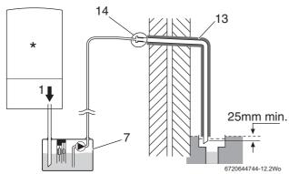
Fig. 9 Condensate pump to external disposal
