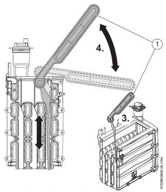
Fig. 74 Cleaning the front channels
