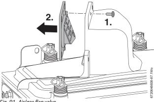
Fig. 91 Air/gas flap valve
