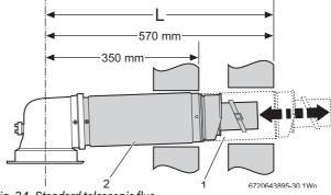
Fig. 34 Standard telescopic flue
