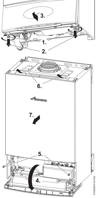
Fig. 76 Removing outer case
