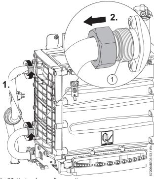
Fig. 97 Heat exchanger disconnection
