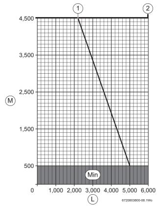
Fig. 19 Effective flue lengths versus plume management lengths
