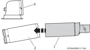
Fig. 35 Reducing the standard terminal
