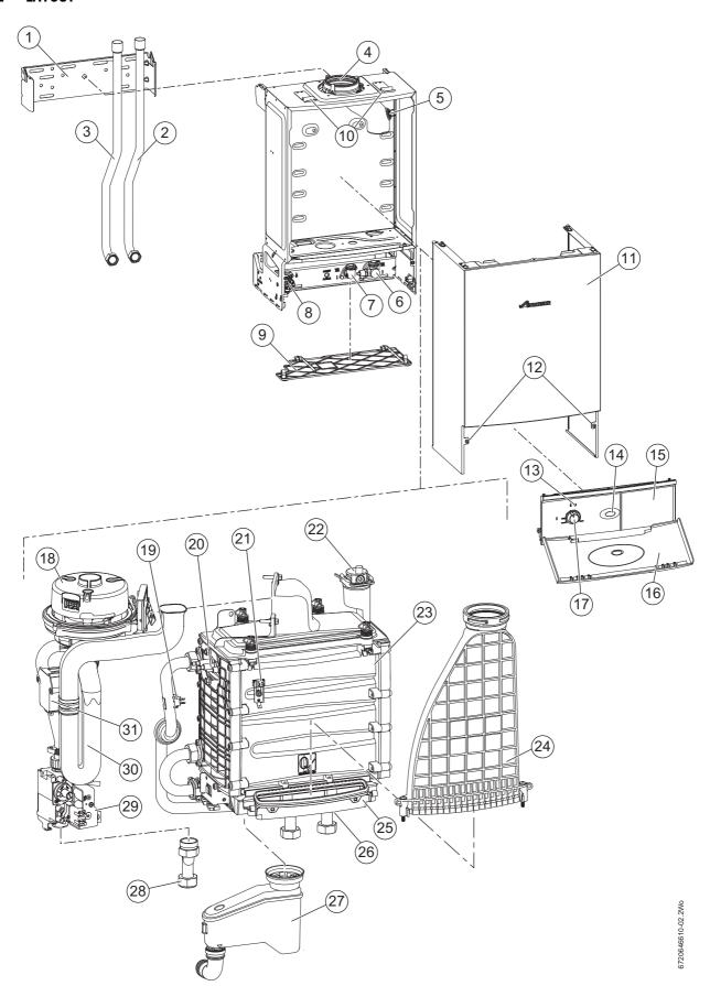
Fig. 2 Ri Compact main boiler components
