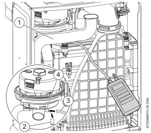
Fig. 66 Fan pressure test point
