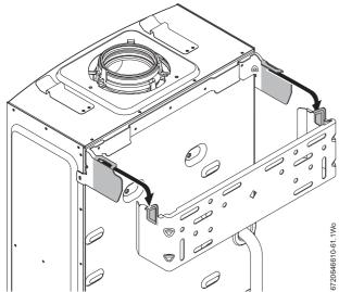
Fig. 29 Hanging the boiler on the wall frame
