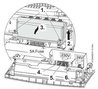
Fig. 43 Removing the installer access cover
