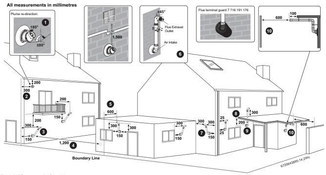
Fig. 16 Plume terminal positions
