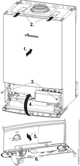
Fig. 59 Fitting case
