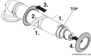
Fig. 37 Telescopic flue
