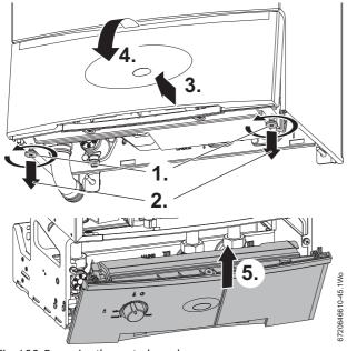
Fig. 100 Removing the control panel
