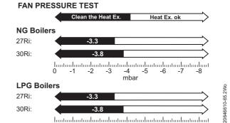
Fig. 67 Fan pressure readings
