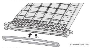
Fig. 87 Tubular style sump seal
