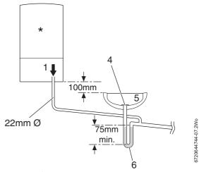
Fig. 5 Disposal to a waste pipe
