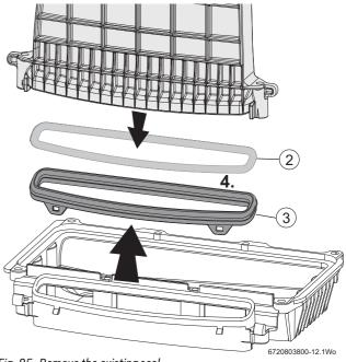
Fig. 85 Remove the existing seal
