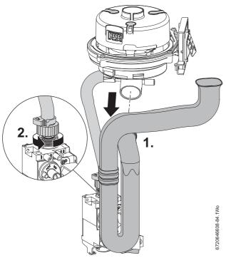
Fig. 88 Combustion air inlet pipe removal
