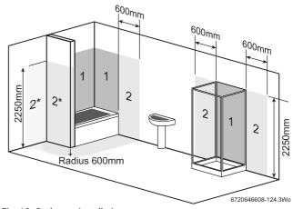
Fig. 12 Bathroom installations
