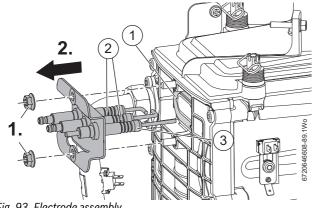
Fig. 93 Electrode assembly
