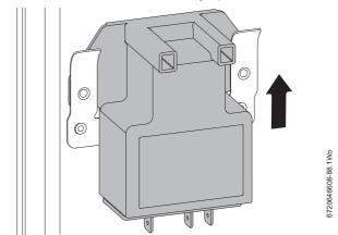
Fig. 92 Ignition transformer
