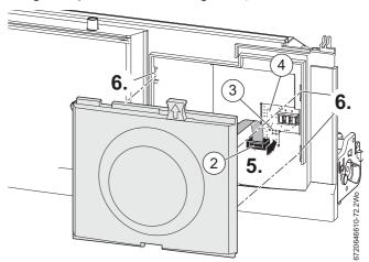
Fig. 46 Connecting the Programmer/Timer
