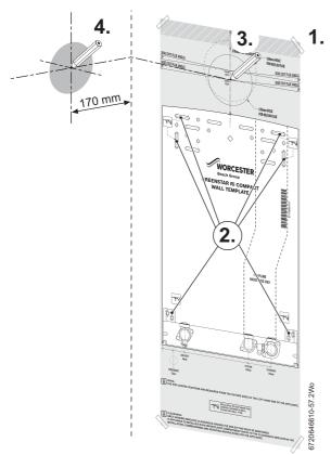
Fig. 22 Marking the flue position
