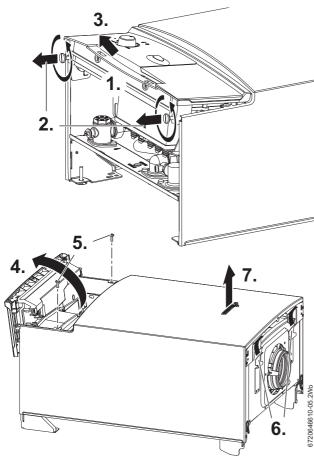
Fig. 25 Releasing the control panel
