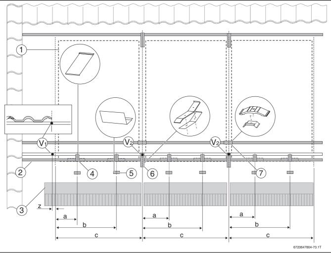
Fig. 40 Installation dimensions for portrait collectors
