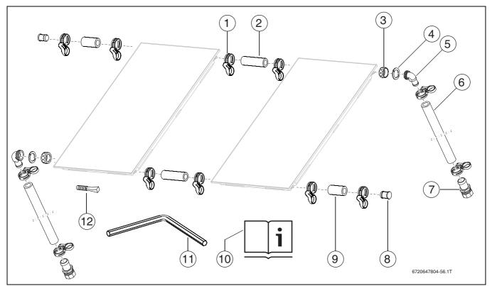
Fig. 14 1 roof integration connection set and 2 interconnection sets
