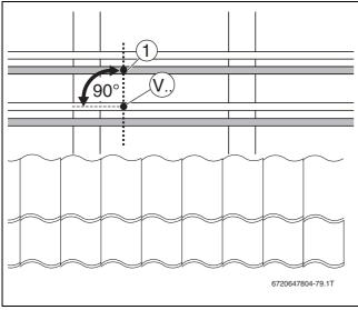
Fig. 43 Transferring reference points
