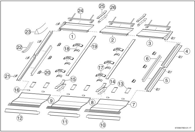
Fig. 5 Installation set for 3 portrait collectors: 1 basic installation set and 1 extension installation set
