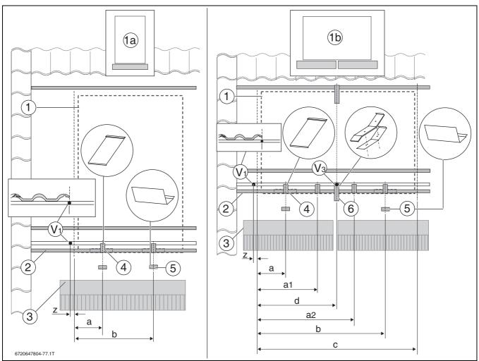
*Fig. 42* Installation dimensions for single collectors
