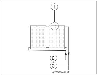
Fig. 65 Position of the collector sensor
