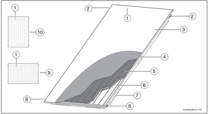
Fig. 1 Cross-section of portrait collector version
