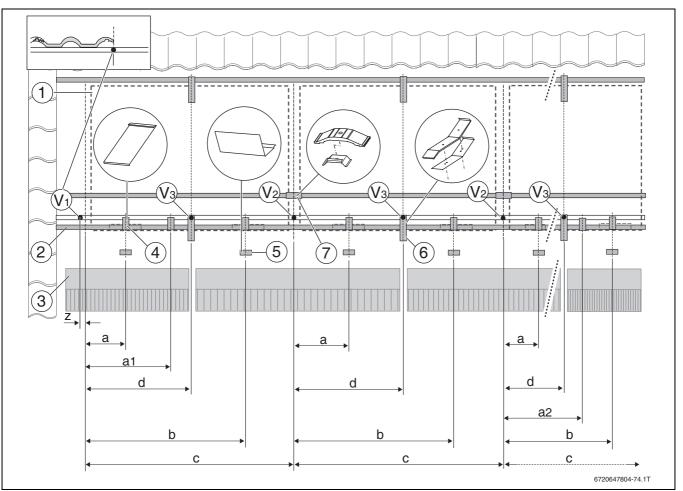
Fig. 41 Installation dimensions for landscape collectors
