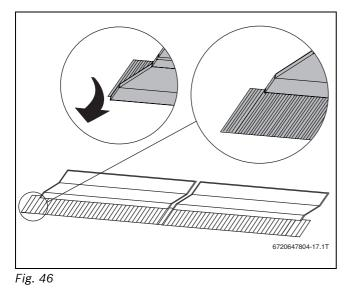
Push the right hand lower flashing panel [1.] into the retainer.
