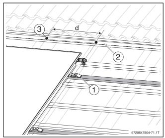
Fig. 57 Installation position of the top joiner for landscape collectors
