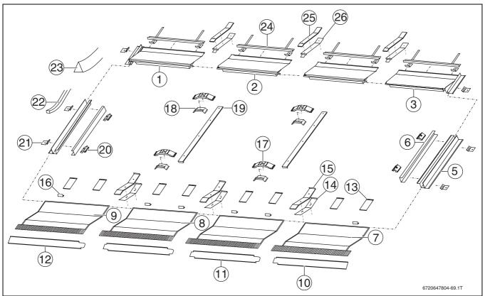
Fig. 8 Installation set for 3 landscape collectors: 1 basic installation set and 1 extension installation set
