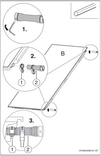
Fig. 34 Interconnection set on the second and all further collectors
