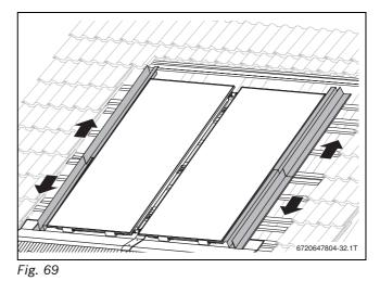
► Secure the flashing panels with 3 mounting brackets.
