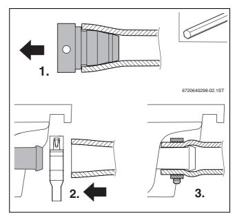
Fig. 31 Installation of the solar hose
