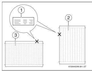
Fig. 3 Data plate position
