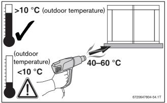
Fig. 84 Heating up the lead flashing at low outdoor temperatures
