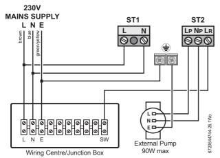
Fig. 40 External wiring centre
