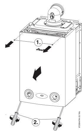
Fig. 71 Remove outer case
