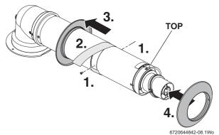
Fig. 33 Telescopic flue
