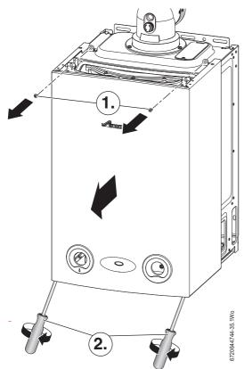
Fig. 52 Remove outer case
