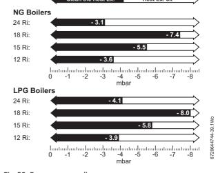
Fig. 58 Fan pressure readings
