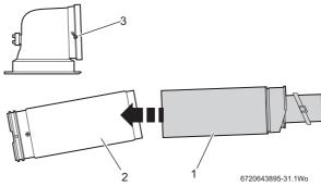
Fig. 32 Reducing the standard terminal
