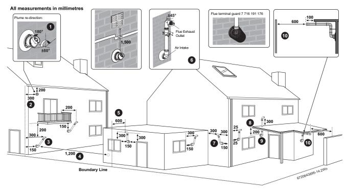
Fig. 21 Plume terminal positions
