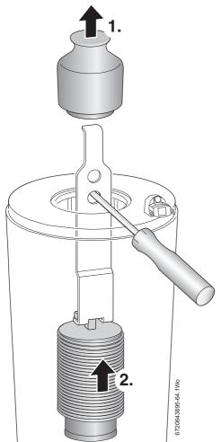
Fig. 66 Baffle removal
