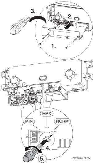
Fig. 56 Setting the boiler to maximum
