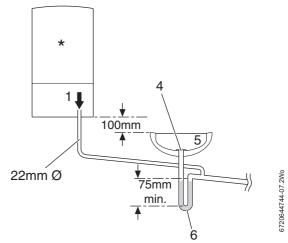
Fig. 9 Disposal to a waste pipe
