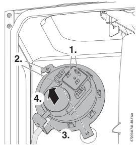
Fig. 80 Air pressure switch
