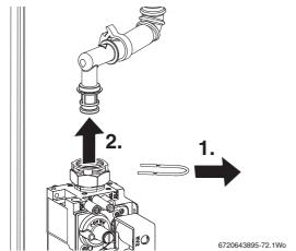
Fig. 76 Gas valve upper connection
