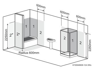
Fig. 17 Bathroom installations
