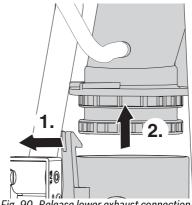
Fig. 90 Release lower exhaust connection
