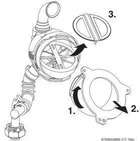
Fig. 83 Flap valve assembly
