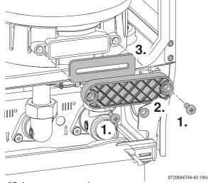
Fig. 67 Access cover removal
