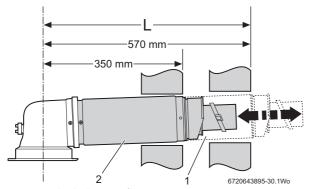
Fig. 31 Standard telescopic flue
