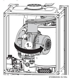
Fig. 79 Rotate the air/gas manifold assembly
