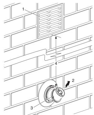
Fig. 38 Plume distance to opening
