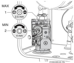
Fig. 61 Gas valve adjustment
