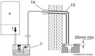
Fig. 14 Condensate pump to external disposal
