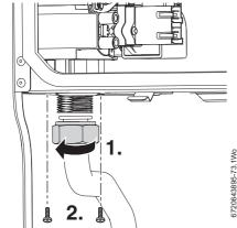
Fig. 77 Gas valve lower connection
