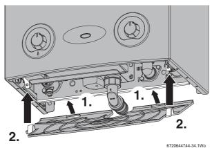
Fig. 70 Remove bottom panel
