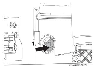
Fig. 74 Remove thermostat
