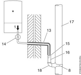
Fig. 11 Disposal into a rainwater down pipe
