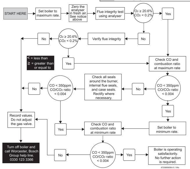
Fig. 49 Combustion check flow chart
