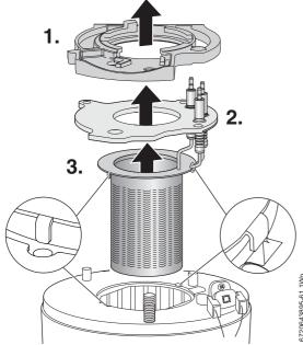
Fig. 84 Electrode assembly and burner
