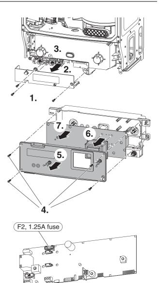
Fig. 96 Change PCB/Fuse location
