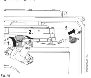
► Undo the securing nut at the top of the heat exchanger and remove the retaining plate assembly (1).
