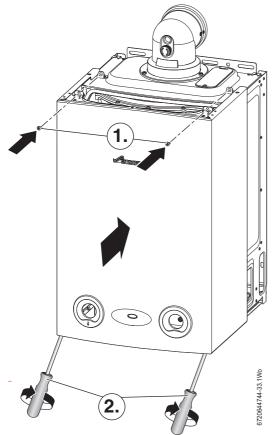
Fig. 50 Replacing outer case
