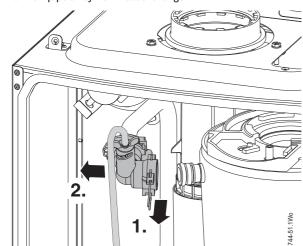
Fig. 88 Flow pipe removal
