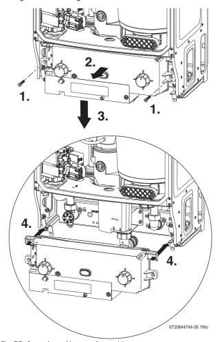
Fig. 75 Control panel into service position
