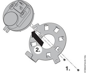
Fig. 81 Air pressure switch bracket
