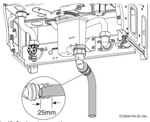
Fig. 43 Condensate connection
