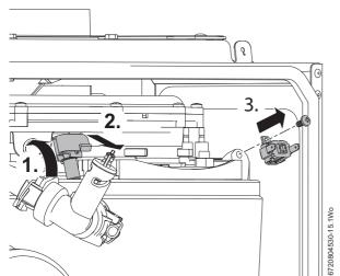
Fig. 72 Primary sensor and overheat thermostat
