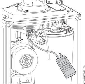
Fig. 57 Fan pressure test
