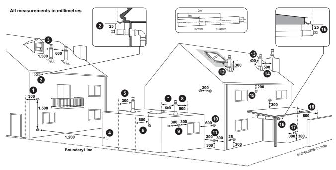
Fig. 20 Flue terminal positions
