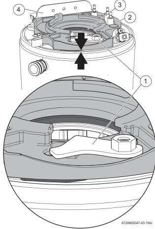
Fig. 85 Initial location of the clamping plate
