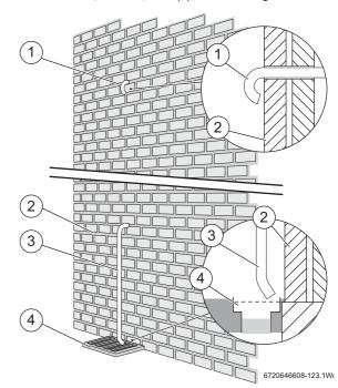
Fig. 15 Pressure relief pipe work
