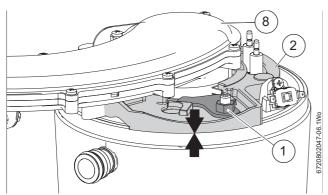
Fig. 87 Clamping plate secured
