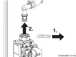
Fig. 62 Gas valve connection
