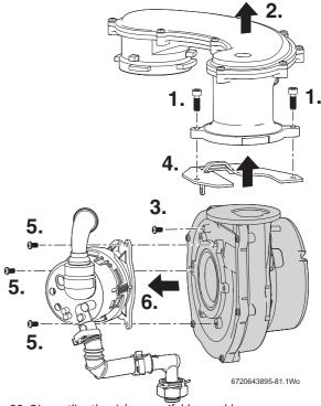
Fig. 82 Dismantling the air/gas manifold assembly
