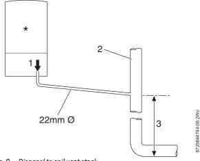
Fig. 8 Disposal to soil vent stack
