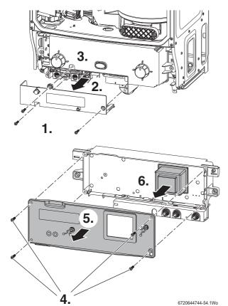
Fig. 95 Transformer/PCB access
