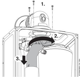
Fig. 89 Upper exhaust assembly
