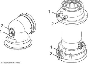
Fig. 54 Flue test points
