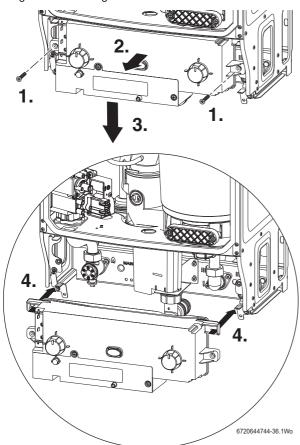
Fig. 53 Control panel into service position
