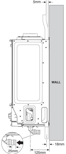
Fig. 29 Pipe work dimensions
