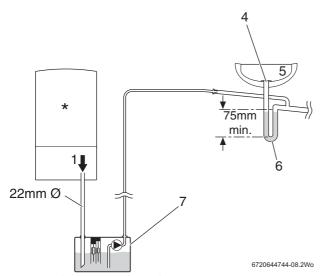
Fig. 10 Condensate pump disposal
