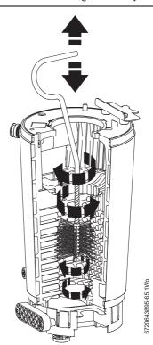
Fig. 68 Cleaning heat exchanger
