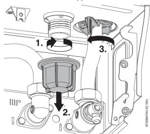
Fig. 91 Sump connections
