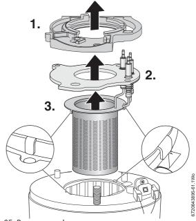
Fig. 65 Burner removal
