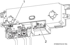
Fig. 94 Removing the connection cover
