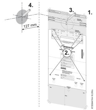
Fig. 24 Marking the flue position
