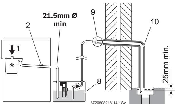
Fig. 13 Condensate pump to external disposal
