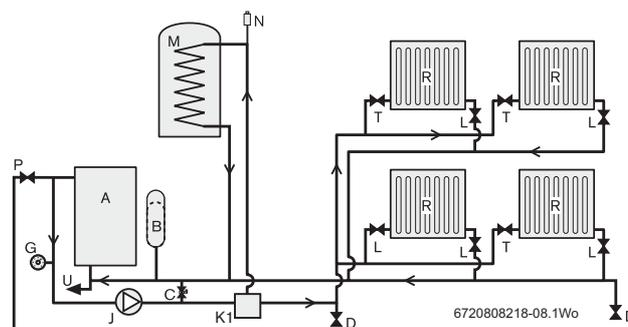
Fig. 6 Regular boiler system layout
