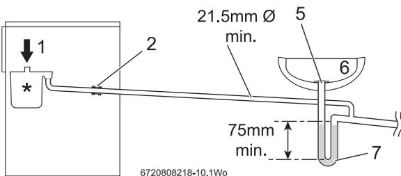
Fig. 9 Disposal to a waste pipe
