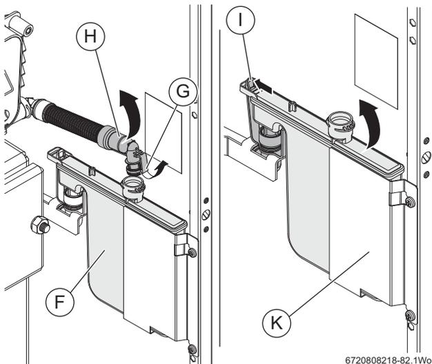
Fig. 79 Condensate trap removal
