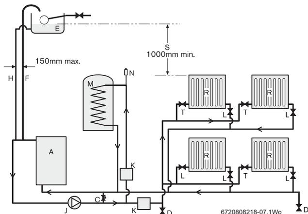
Fig. 5 Regular boiler, open vent system layout
