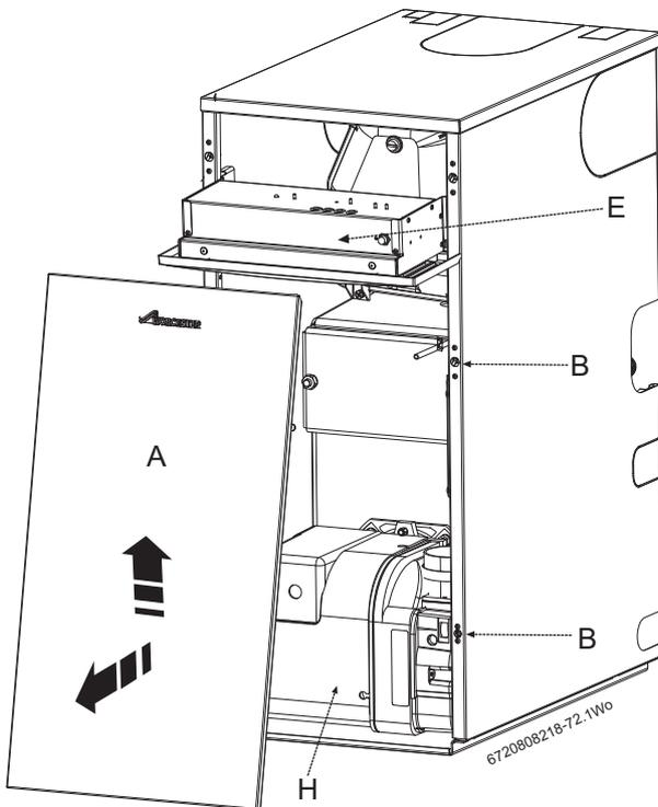
Fig. 69 Access to internal components
