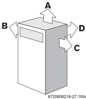
Fig. 32 Flue outlet options
