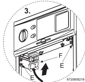
Fig. 46 Refitting the control panel
