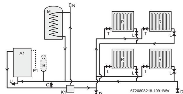
Fig. 7 System boiler system layout
