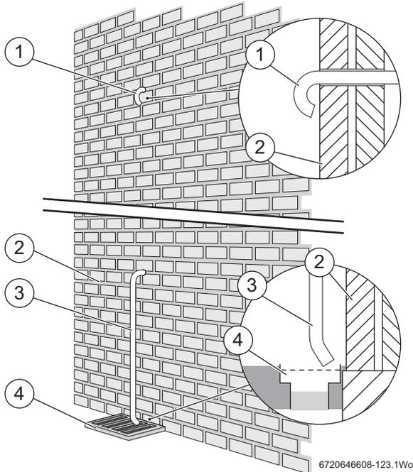
Fig. 15 Pressure relief pipe work
