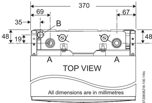
Fig. 23 Top view of Regular boiler pipe connections
