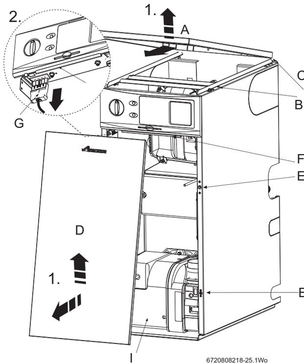
Fig. 29 Boiler installation
