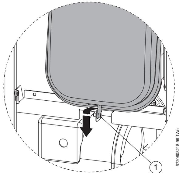
Fig. 70 Expansion vessel removal
