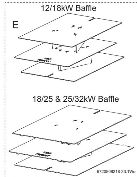
Fig. 38 Baffle arrangement
