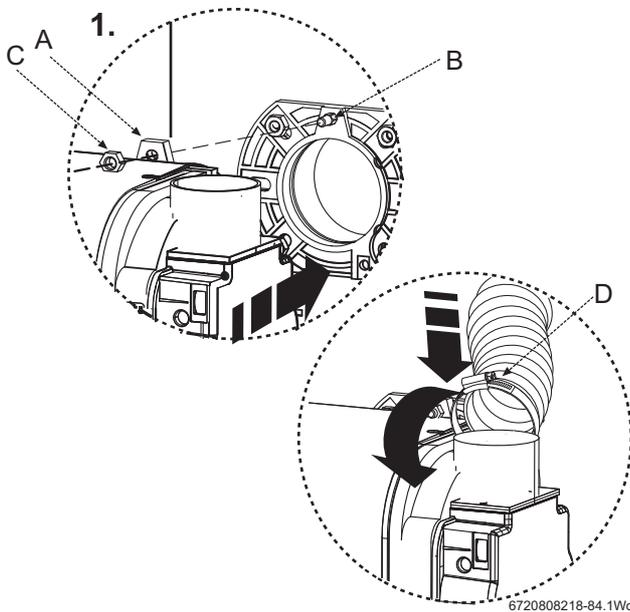
Fig. 81 Refitting the burner
