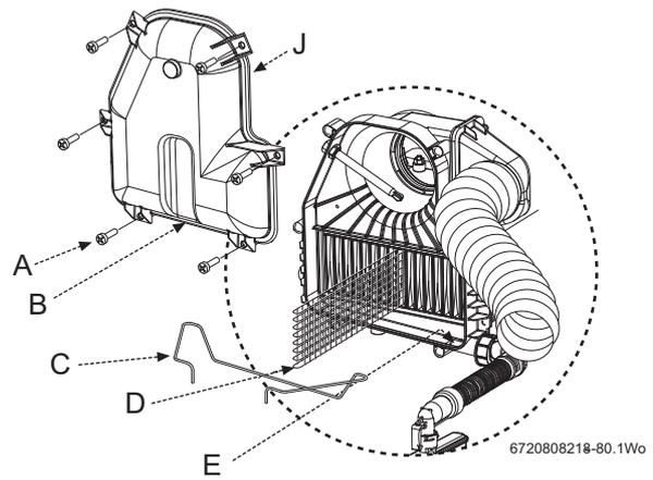
Fig. 80 Heat exchanger baffles
