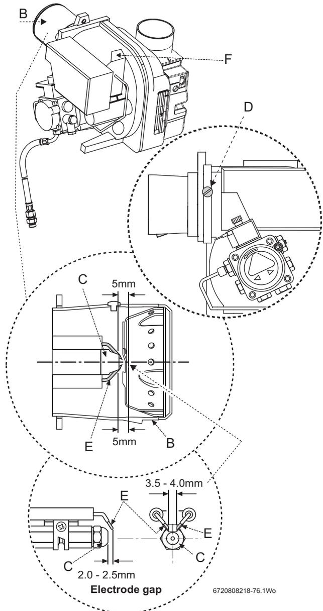
Fig. 74 Burner removal
