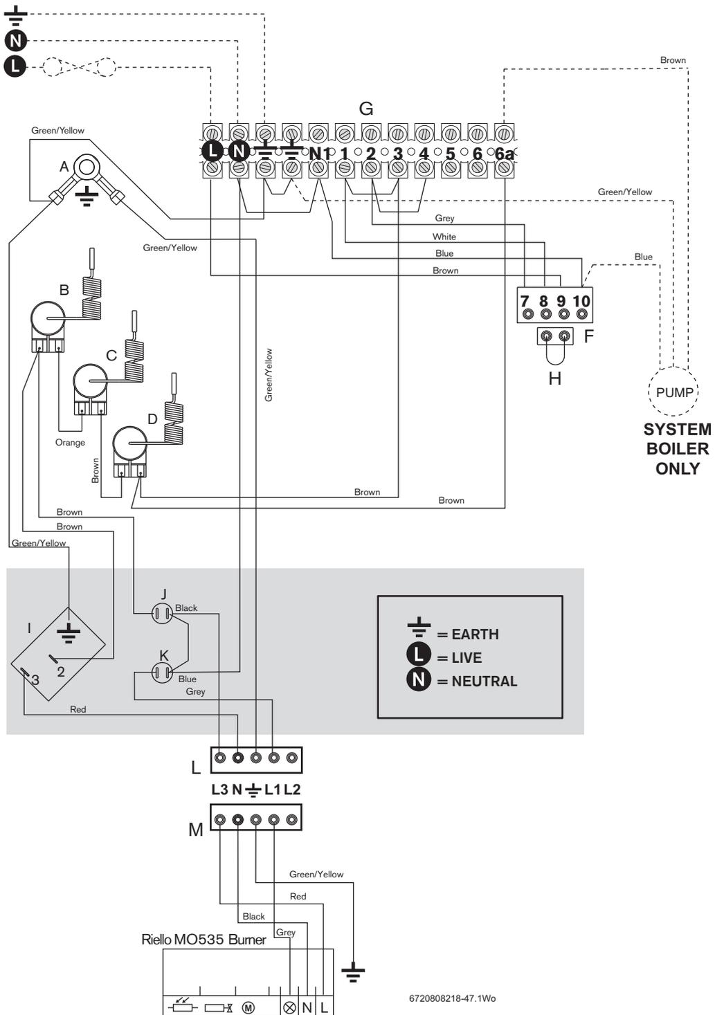
Fig. 50 230V Standard wiring diagram
