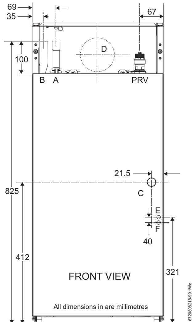
Fig. 26 Front view of System boiler pipe connections
