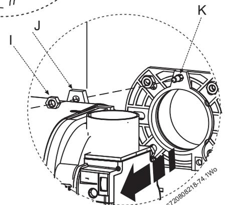
Fig. 72 Burner removal
