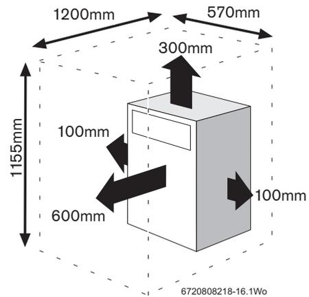
Fig. 16 Installation clearances
