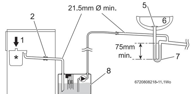
Fig. 10 Disposal via a condensate pump
