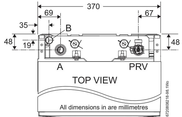
Fig. 25 Top view of System boiler pipe connections
