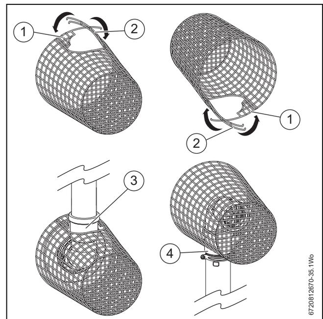
Fig. 37 Fitting terminal guard
