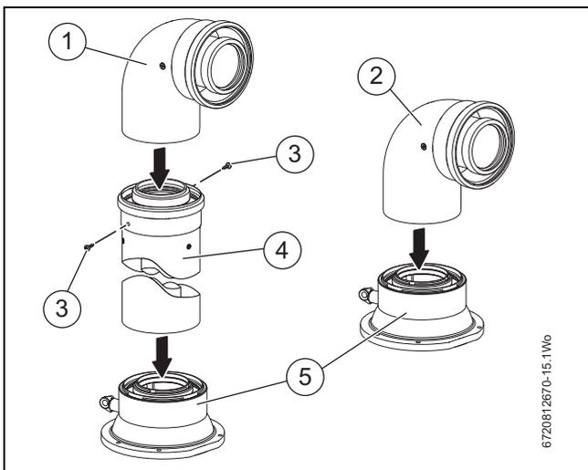
Fig. 16 Connection to the flue adaptor examples
