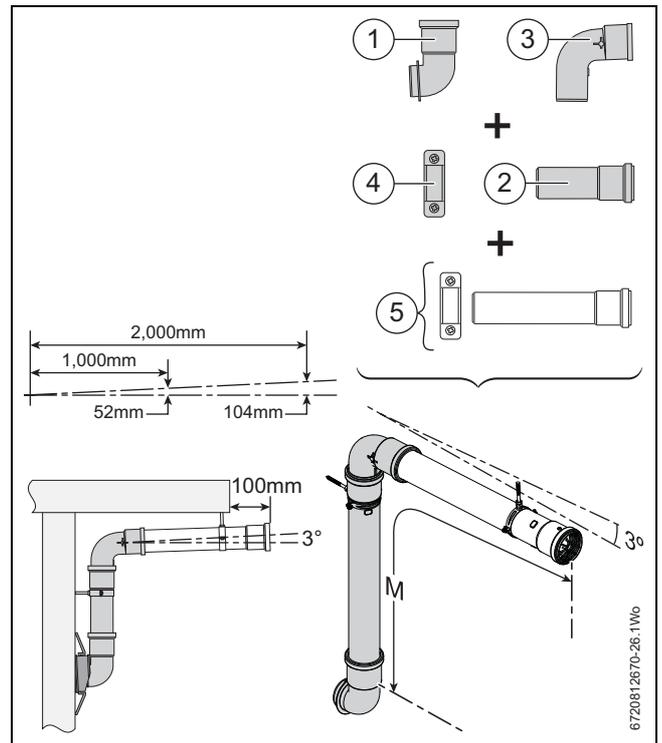
Fig. 28 Extended under a balcony/overhang option
