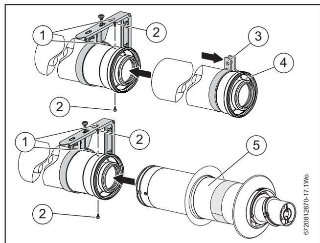
Fig. 18 Extension and telescopic flue connection examples
