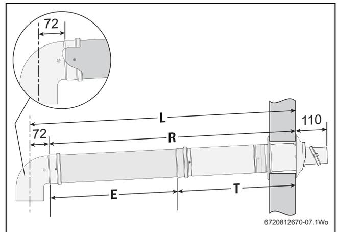
Fig. 6 Flue length determination (extended flue example)
