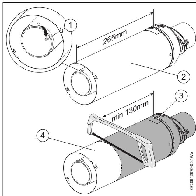
Fig. 11 Shortening the terminal assembly
