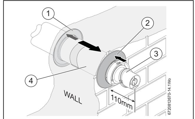
Fig. 14 Telescopic flue through the wall
