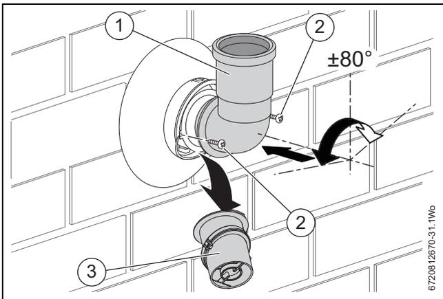
Fig. 33 Plume management terminal bend
