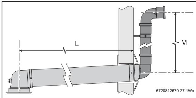
Fig. 29 Effective lengths determination
