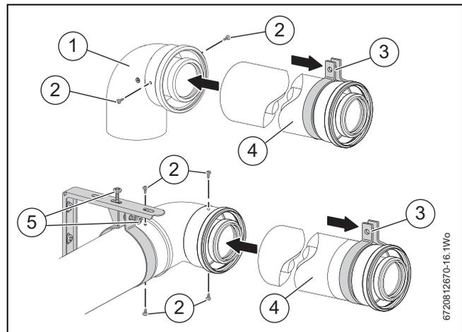
Fig. 17 Elbow connection examples (90° bend)
