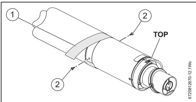
Fig. 13 Setting the telescopic flue length
