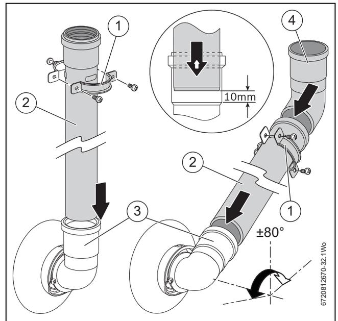
Fig. 34 Plume extension fitting
