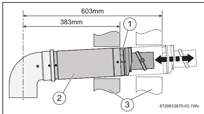
Fig. 9 Standard telescopic flue lengths
