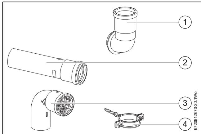
Fig. 21 60mm plume management kit components
