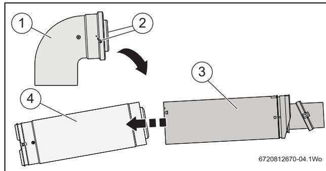
Fig. 10 Separating elbow from telescopic flue
