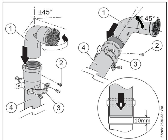
Fig. 35 Fitting the discharge elbow
