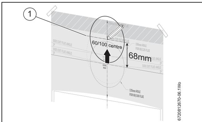
Fig. 5 Adjusted 60/100mm flue exit hole
