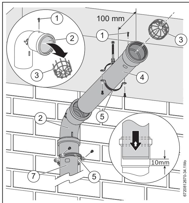
Fig. 36 Fitting extension under balcony/overhang
