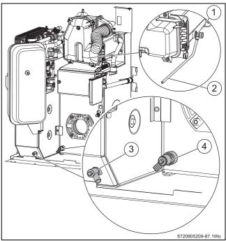
Fig. 72 Appliance drains points
