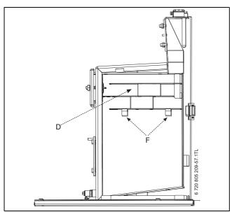
Fig. 81 Baffle location
