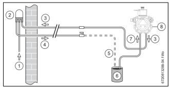
Fig. 57 Priming the pump
