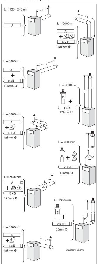
Fig. 24 Room seal ed flue options
