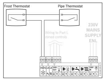
Fig. 46 Optional External 230 VAC Frost Stat Connection for protection of system pipework in unheated air space
