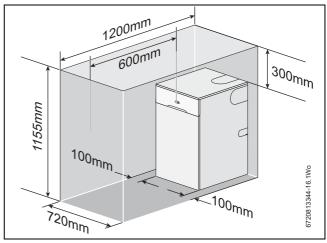
Fig. 19 Installation clearances
