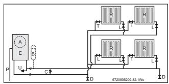
Fig. 8 Combi boiler sealed system layout
