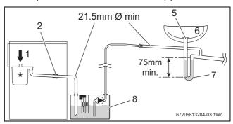
Fig. 13 Disposal via a condensate pump
