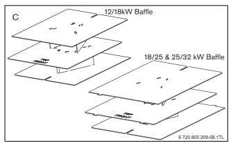
Fig. 80 Baffle arrangement
