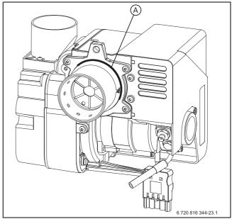
Fig. 82 Burner O-ring seal
