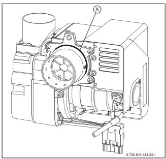
Fig. 39 Burner O-ring seal
