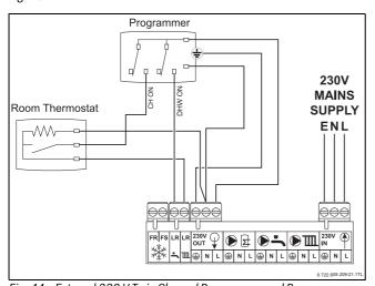
Fig. 44 External 230 V Twin Channel Programmer and Room Thermostat
