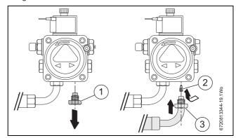
Fig. 38 Converting to double pipe system
