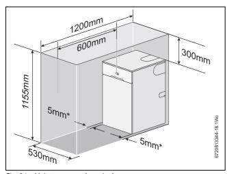
Fig. 21 Maintenance and repair clearances
