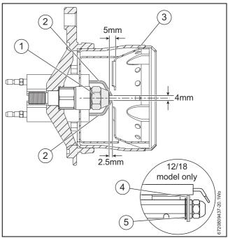
Fig. 37 Nozzle and electrode alignment
