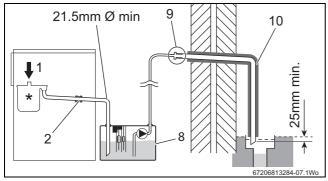
Fig. 16 Condensate pump to external disposal
