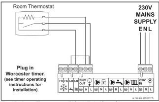
Fig. 45 Room Thermostat and Plug In Twin Channel Programmer
