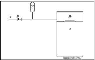
Fig. 3 Mains expansion vessel
