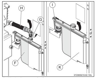
Fig. 78 Condensate trap detail
