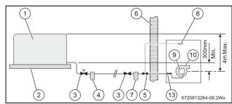
Fig. 4 Single pipe feed
