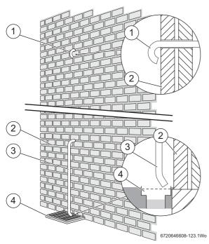
Fig. 18 Pressure relief pipe work
