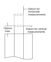
The datum for vertical measurements is the point of discharge of the flue, or 150mm above the insulation, whichever is the lower
