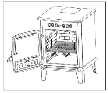
Slide the log retainer down into the slots located at the front of the door
