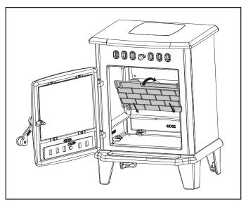
Next install the wood grate. Note that there are two small notches and two large notches. The two large notches must face to the front of the stove or the grate will not correctly install.
