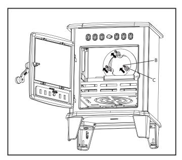
Reach in through the front door of the stove and remove the three (B) bolts, and (C) washers, that are holding on the flue collar.
