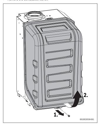
Fig. 62 Removing the combustion cover
