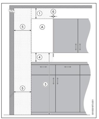
Fig. 11 Reduced front maintenance clearances - Front view
