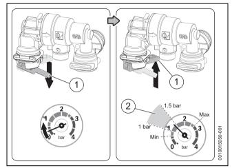
Fig. 5 Keyless filling link
