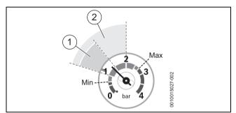
*Fig. 2 Pressure gauge for checking the operating pressure*
