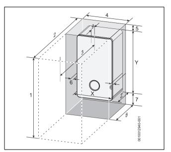
Fig. 9 Appliance minimum clearances
