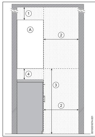
Fig. 10 Reduced front maintenance clearances - Side view
