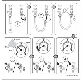
Fig. 4 External filling loop
