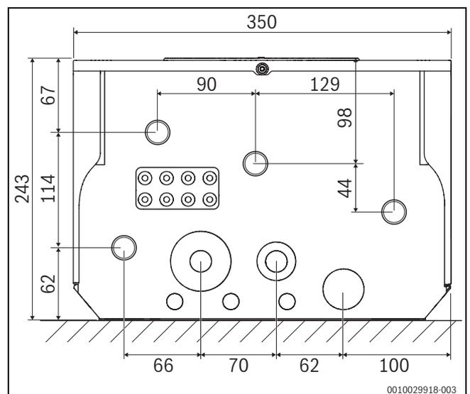
Fig. 5 Clearances between connections (mm)
