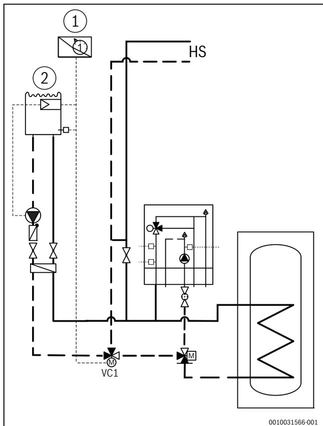
Fig. 23 Example showing swimming pool installation
