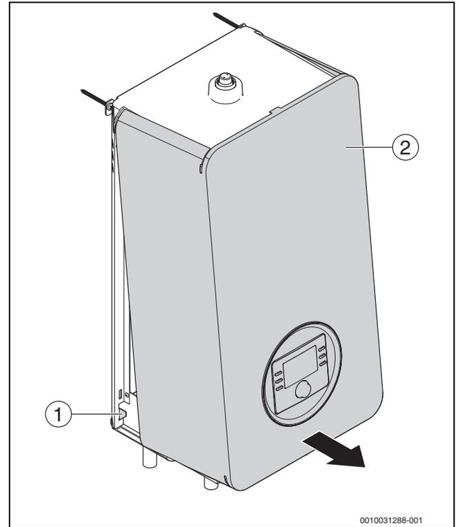
Fig. 12 Detach the cover from the bottom fixing
