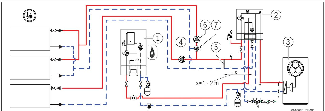
Fig. 43 Hydraulic diagram of a system (2 heating circuits, with bypass and heating pump; example)
