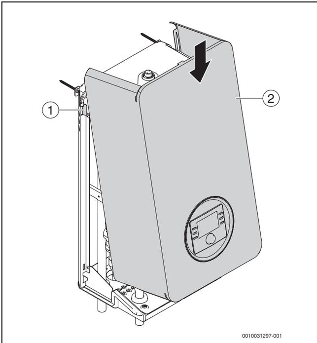
Fig. 17 Attach the cover to the top fixing
