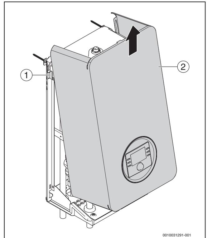
Fig. 13 Detach the cover from the top fixing
