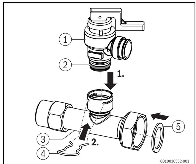
Fig. 7 Assembly of the pressure-relief valve
