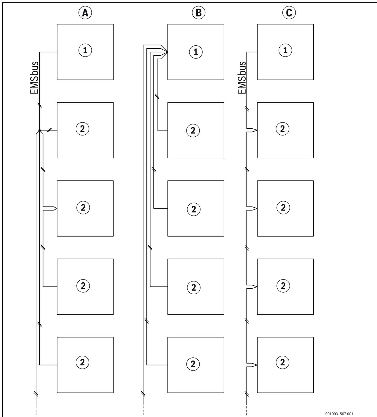
Fig. 32 Connection alternative for EMS bus
