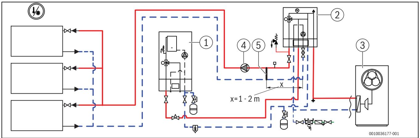
Fig. 42 Hydraulic diagram of a system (1 heating circuit, with bypass and heating pump), with bypass and heating pump; example)
