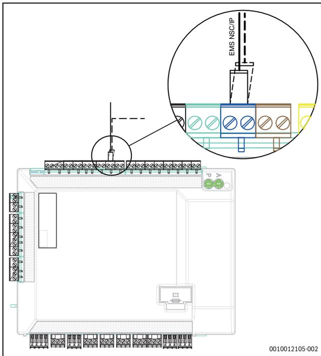
Fig. 31 EMS connection on the installer module
