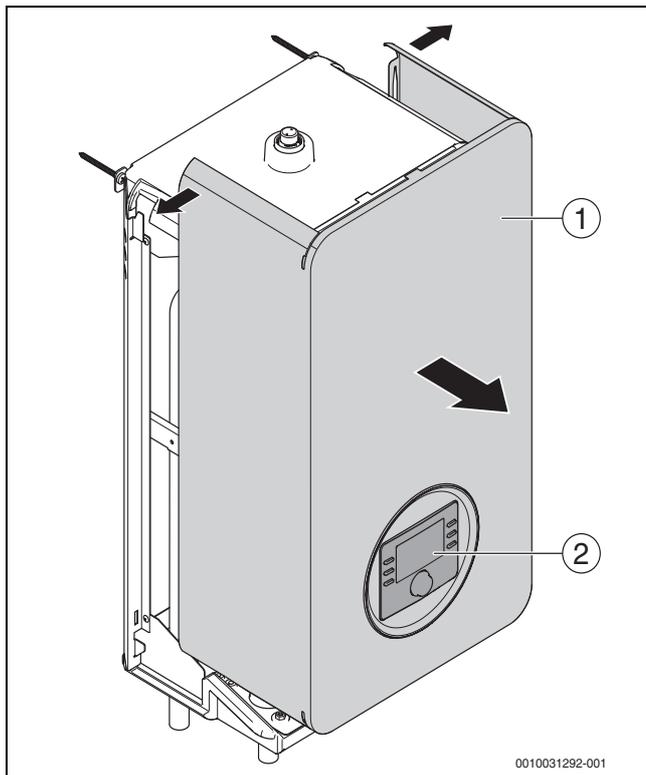
Fig. 14 Removing the cover
