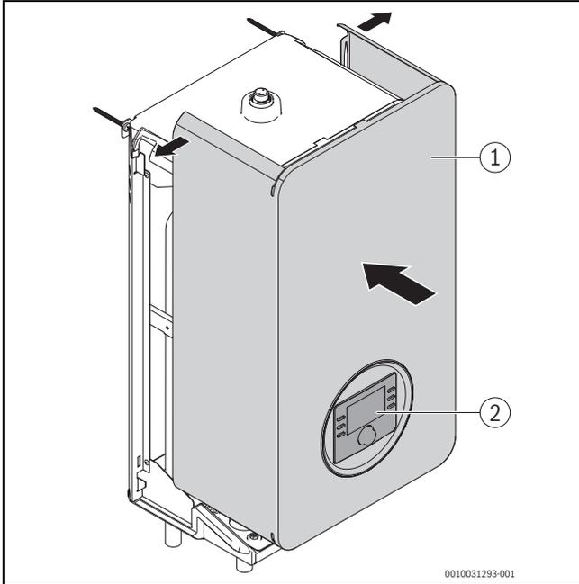
Fig. 16 Fitting the cover
