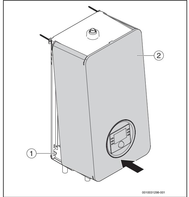
Fig. 18 Attach the cover to the bottom fixing
