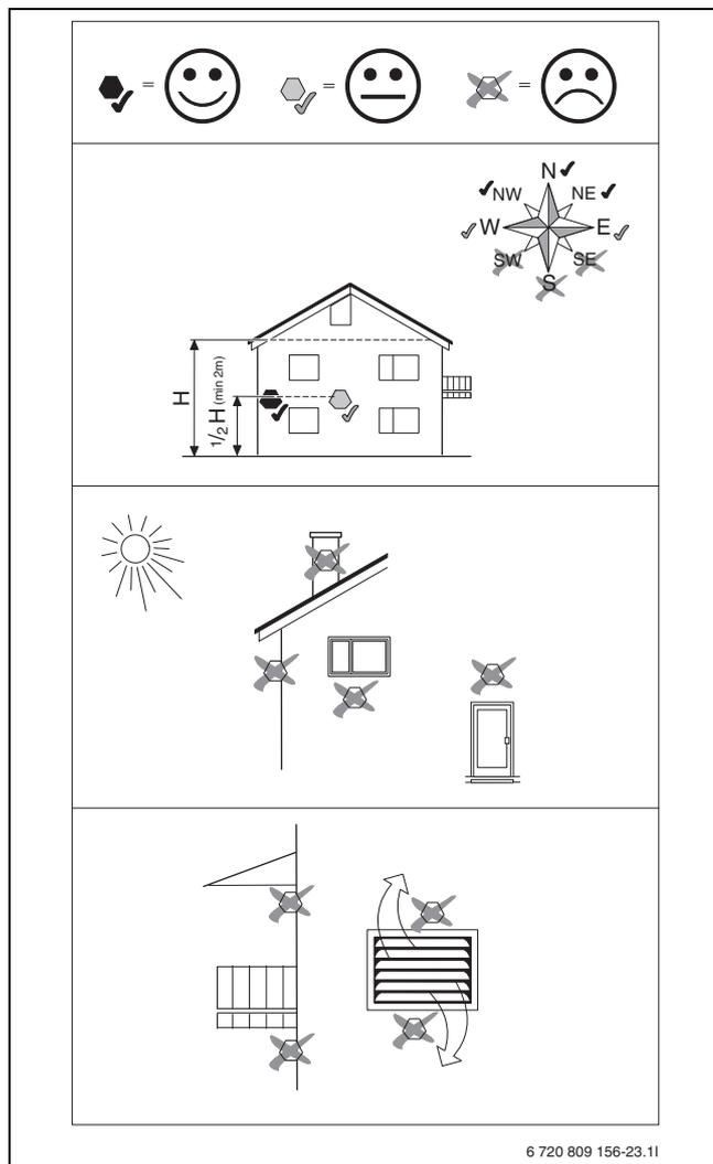
Fig. 22 Positioning the outside temperature sensor
