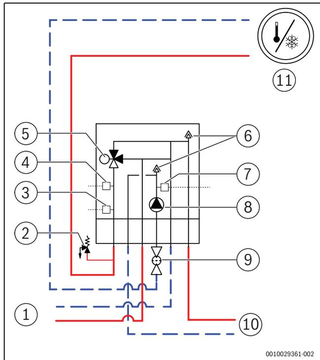
Fig. 40 Hydraulic diagram of the indoor unit
