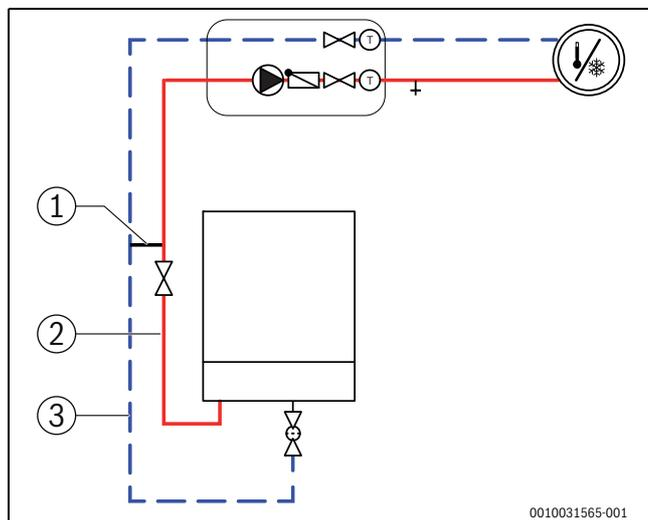
Fig. 8 Indoor unit with heating circuit and bypass
