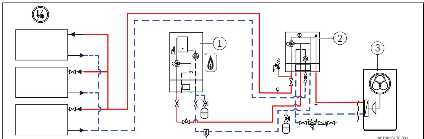
Fig. 41 Hydraulic diagram of a system (1 heating circuit, without bypass; example)
