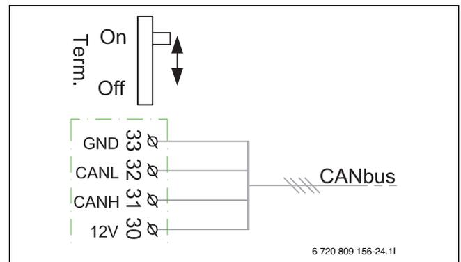
Fig. 27 Termination CAN-BUS
