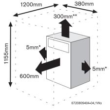
Conventional flue boilers require an adequate supply of fresh air which must be delivered to the boiler for combustion purposes through a permanent inlet, such as an air brick, into the area where the boiler is situated.
