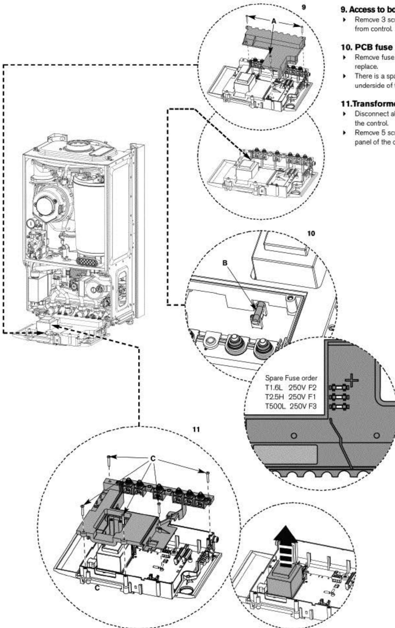
**9. Access to boiler control components**
