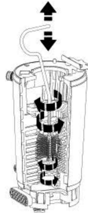
Clean around sealing surface on sump and replace access cover (Q). Using a suitable container to collect water from syphon connection at the base of the boiler flush heat exchanger with water.
