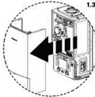
**2. Adjusting boiler control to service position**
