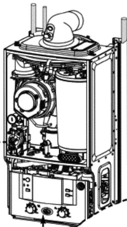
**NOTE:** When running in the service mode, the boiler will operate both the central heating and the domestic hot water circuits. This is to allow sufficient time for this part of the commissioning procedure. It will be necessary to run water through the domestic hot water circuit to ensure that the boiler will not cycle on low heating demands.
