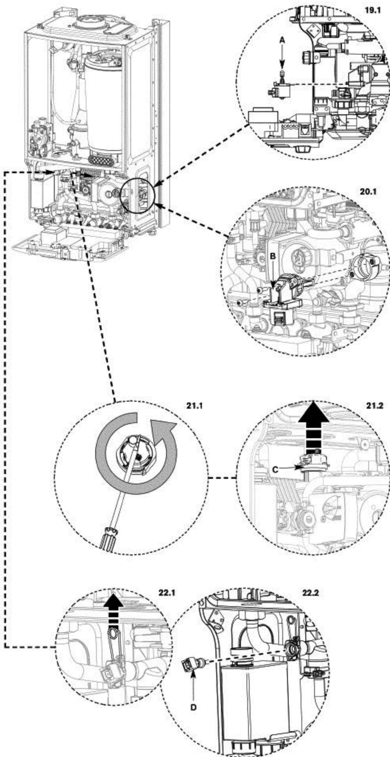
**19. Diverter valve motor**
