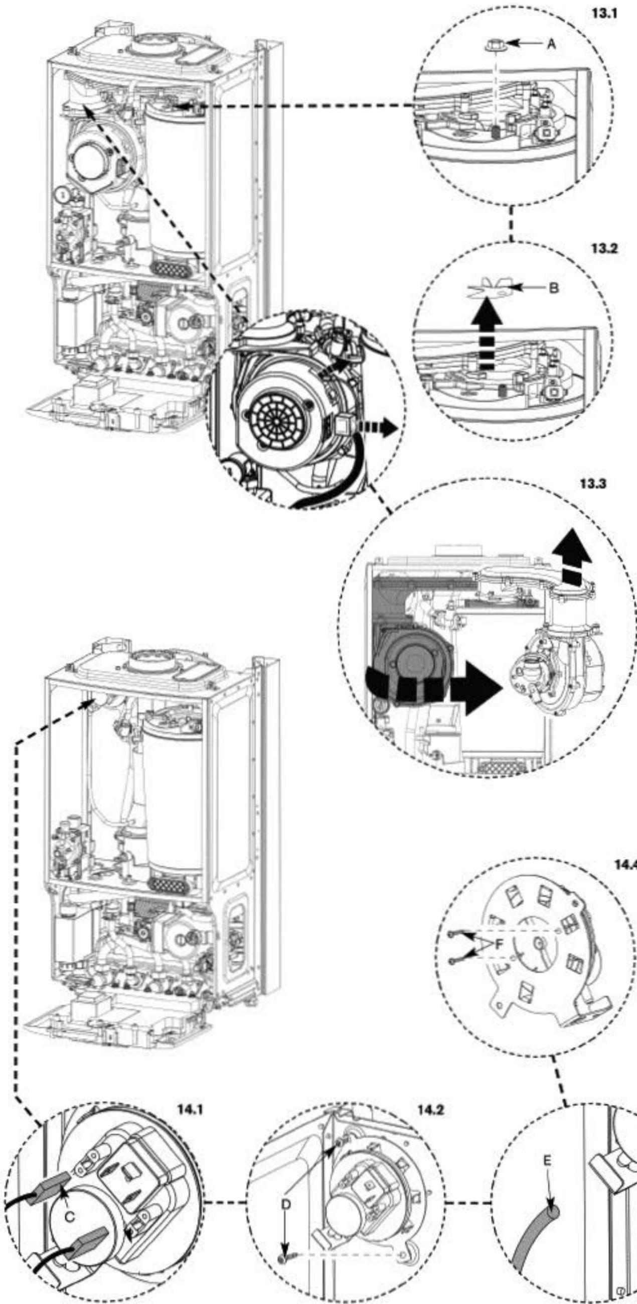
The following components require the air / gas manifold and fan assembly to be removed:
