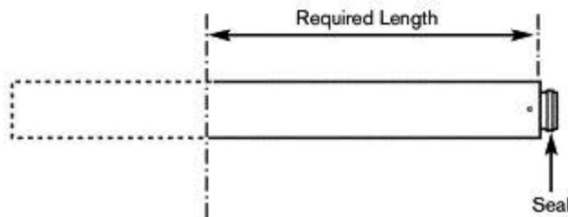
NOTE: Where extensions are reduced, cut length which **DOES NOT** contain the seal.
