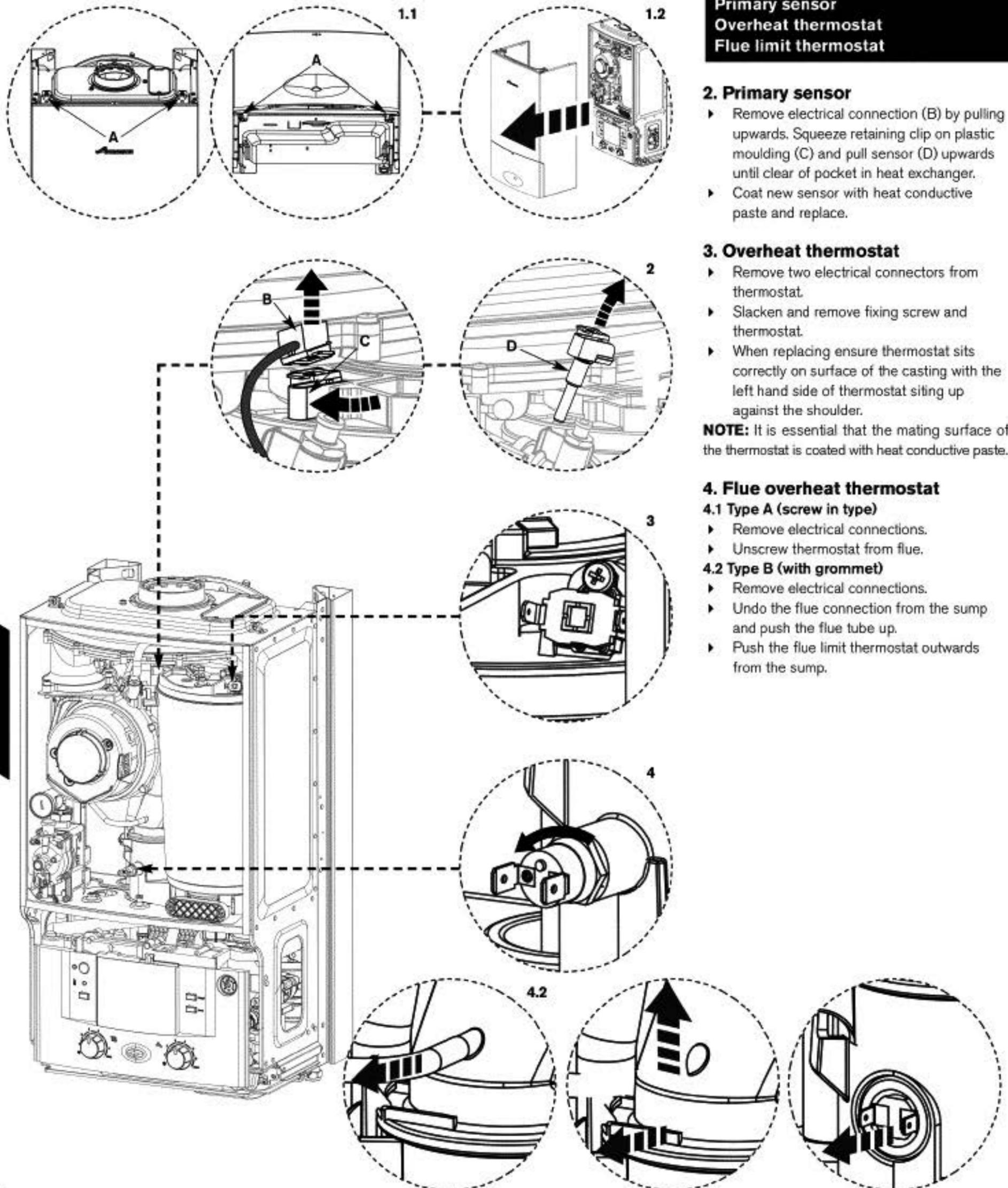
The following components require the control to be moved in to the service position:
