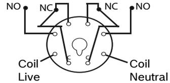
Example relay shown is a double Pole Mains Voltage Relay. This disables the boilers electrically in case of a fault condition.
